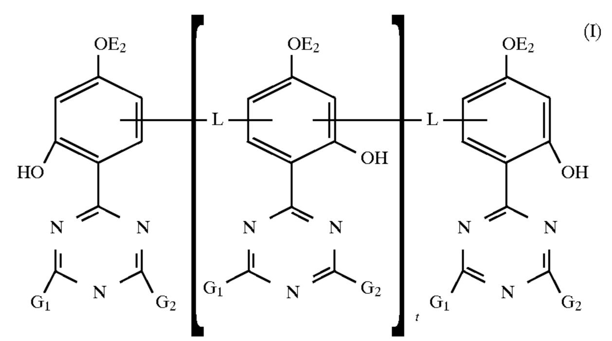
where  $G_1$  and  $G_2$  are biphenylyl moieties, are UV absorbers having high thermal stability and surprisingly high extinction coefficients making them of especial interest in stabilizing automotive coatings where such properties are highly valued.
