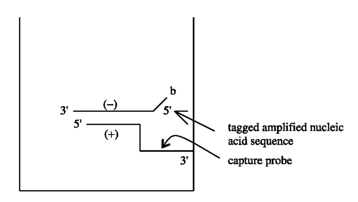
The reaction mixture is cooled, preferably to optimal annealing temperature, thus resulting in the tagged amplified nucleic acid sequence being captured by the capture probe (via standard AT and GC pairings, and including non standard pairings). Non-captured materials are then washed out of the reaction vessel.
