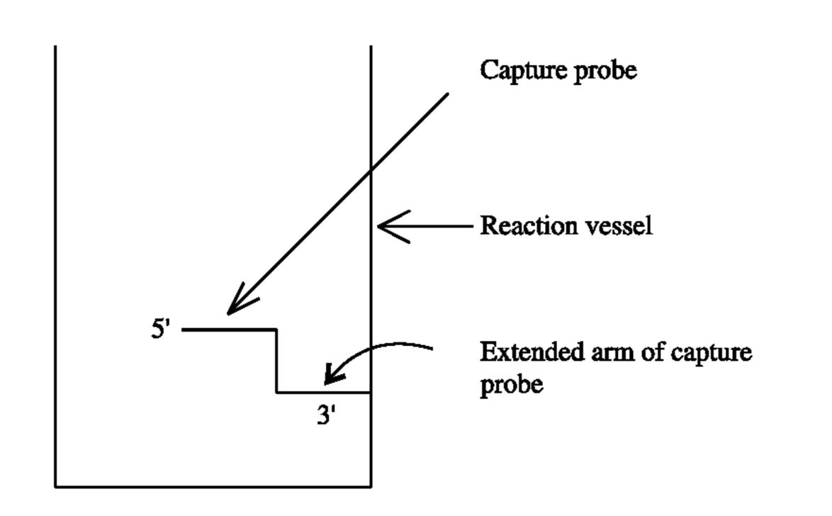
The reaction vessel comprises a solid phase capture probe which is incapable of participation in nucleic acid amplification. For example, the capture probe is covalently linked to the inside surface or wall of the reaction vessel via its 3'-end, or the 3'-end is modified such that it cannot participate in polymerase mediated amplification. The 5'-end lacks a phosphate and, therefore, the capture probe cannot participate in LCR (ligase chain reaction).
