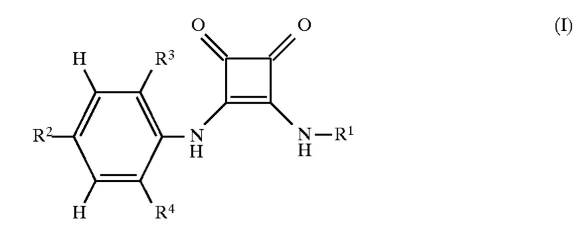
wherein R<sup>1</sup> is straight chain alkyl, branched chain alkyl, cycloalkyl, hydroxyalkyl, fluoroalkyl, or polyfluoroalkyl; and one of R<sup>2</sup>, R<sup>3</sup> and R<sup>4</sup> is hydroxyl and the other two are, independently, H, CN, halogen, alkyl or hydroxyl; or a pharmaceutically acceptable salt thereof, is useful as a smooth muscle relaxant.
