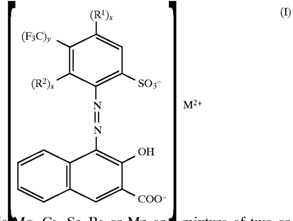
where M is Mg, Ca, Sr, Ba or Mn or mixture of two or more thereof, R<sup>1</sup> and R<sup>2</sup> are chlorine or methyl, x is zero or 1, y is zero or 1 and the sum of x and y is 1, with the proviso that when the high molecular weight material is polyvinyl chloride y is zero.
