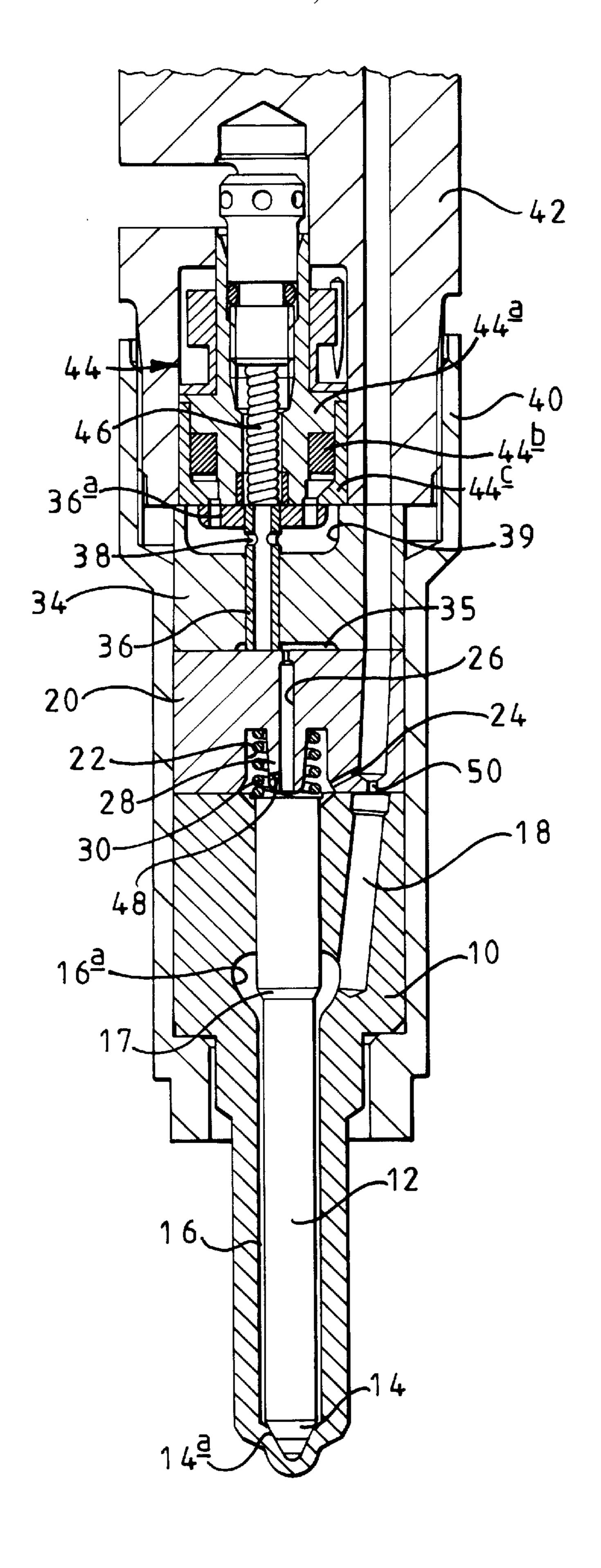
This invention relates to an injector, in particular to an injector for use in a common rail injector arrangement.
