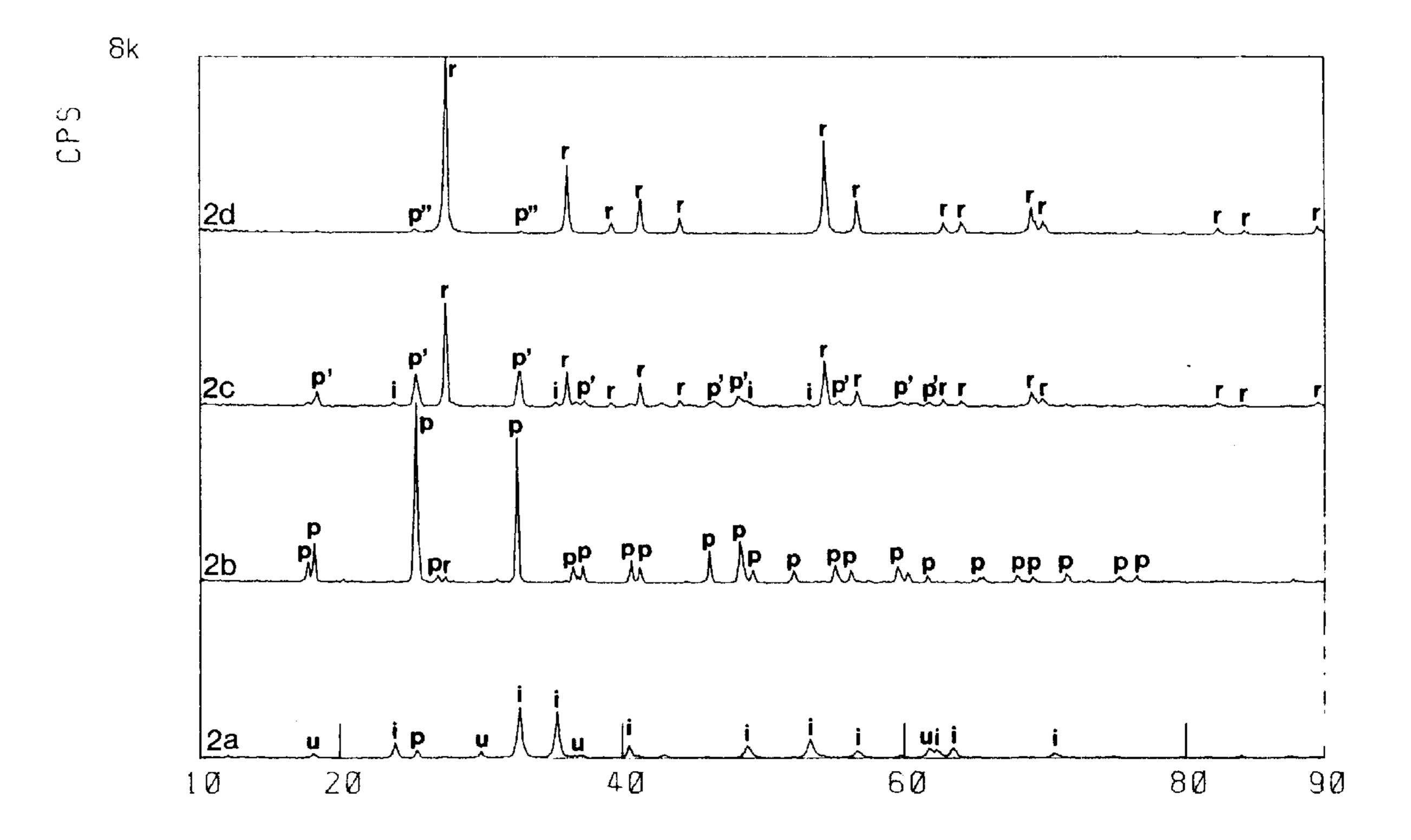
Figure 2 - X-ray diffraction patterns of roasted Allard Lake ilmenite ore (2a), Sorelslag (2b), oxidized/reduced Sorelslag (2c) and UGS product (2d).i - ilmenite, u-ulvospinel, p-ferrous pseudobrookite, r-rutile,
