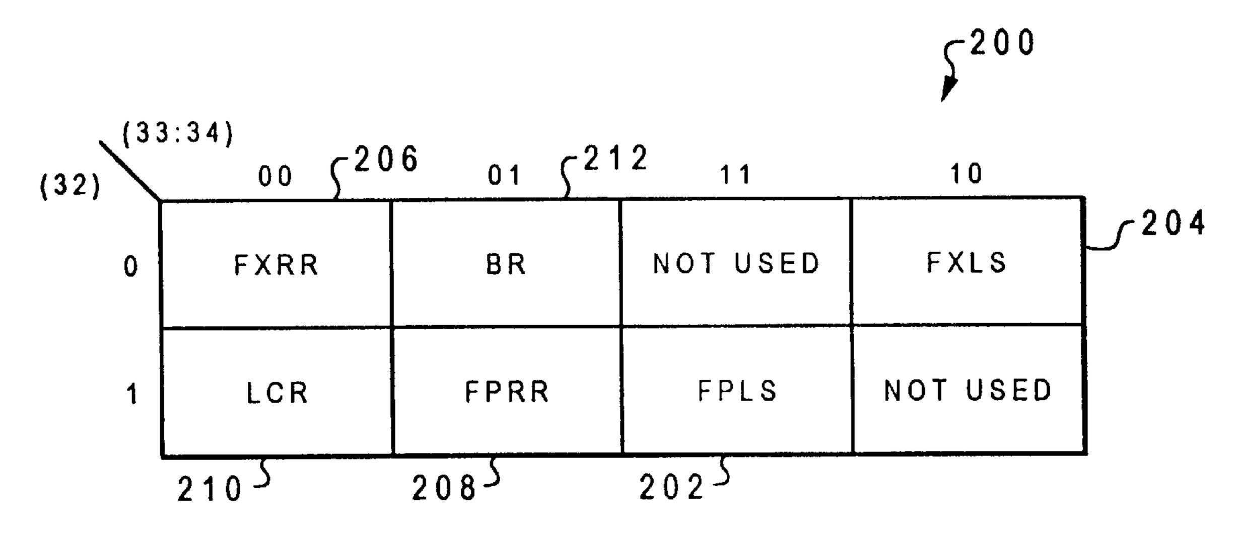
Bit (35..37) - Buffer targets and CR target decode
