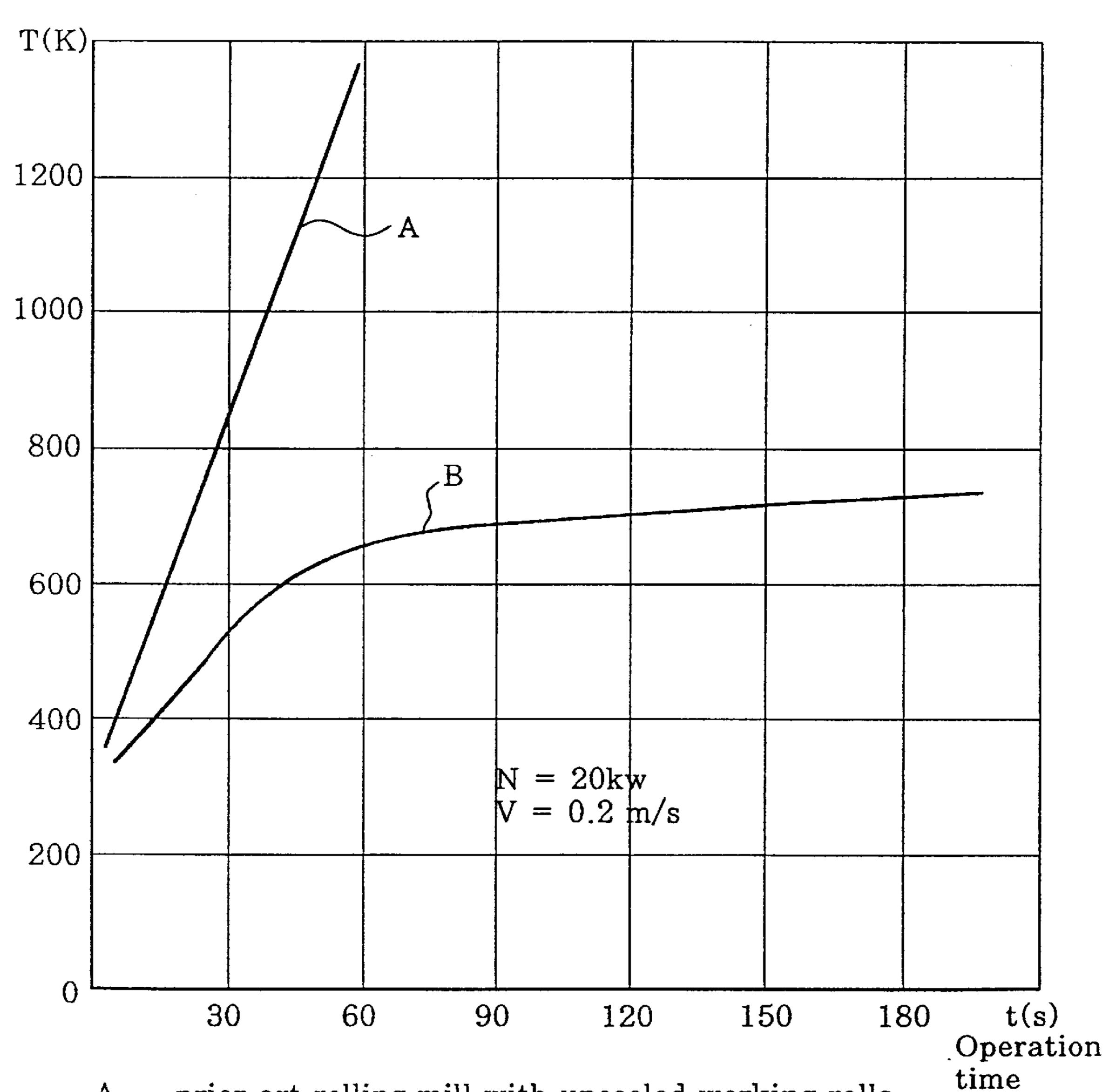
A - prior art rolling mill with uncooled working rolls.
