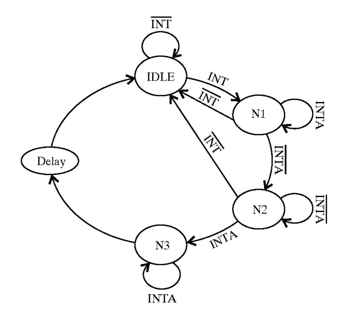
wherein when the state machine is in the N1, N2 and N3 states the state machine circuitry outputs an edge sensitive interrupt signal, when the state machine is in the Delay state the state machine circuitry outputs no interrupt signal, the INT signal comprising an active result of the logical OR of the interrupt lines from the agents on the first I/O bus, the INTA signal comprising a signal from the CPU indicating that it is processing an interrupt.
