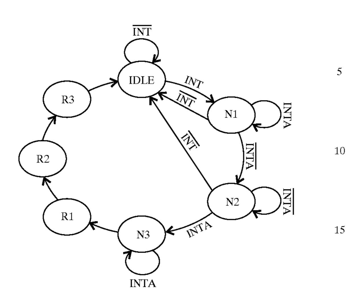
wherein when the state machine is in the N1, N2 and N3 states the state machine circuitry outputs an edge sensitive interrupt signal, the INT signal comprising an active result of the logical OR of the interrupt lines from the agents on the first I/O bus, the INTA signal comprising a signal from the CPU indicating that it is processing an interrupt, the R1, R2 and R3 states comprising successive state machine states where the state machine circuitry outputs no interrupt signal.
