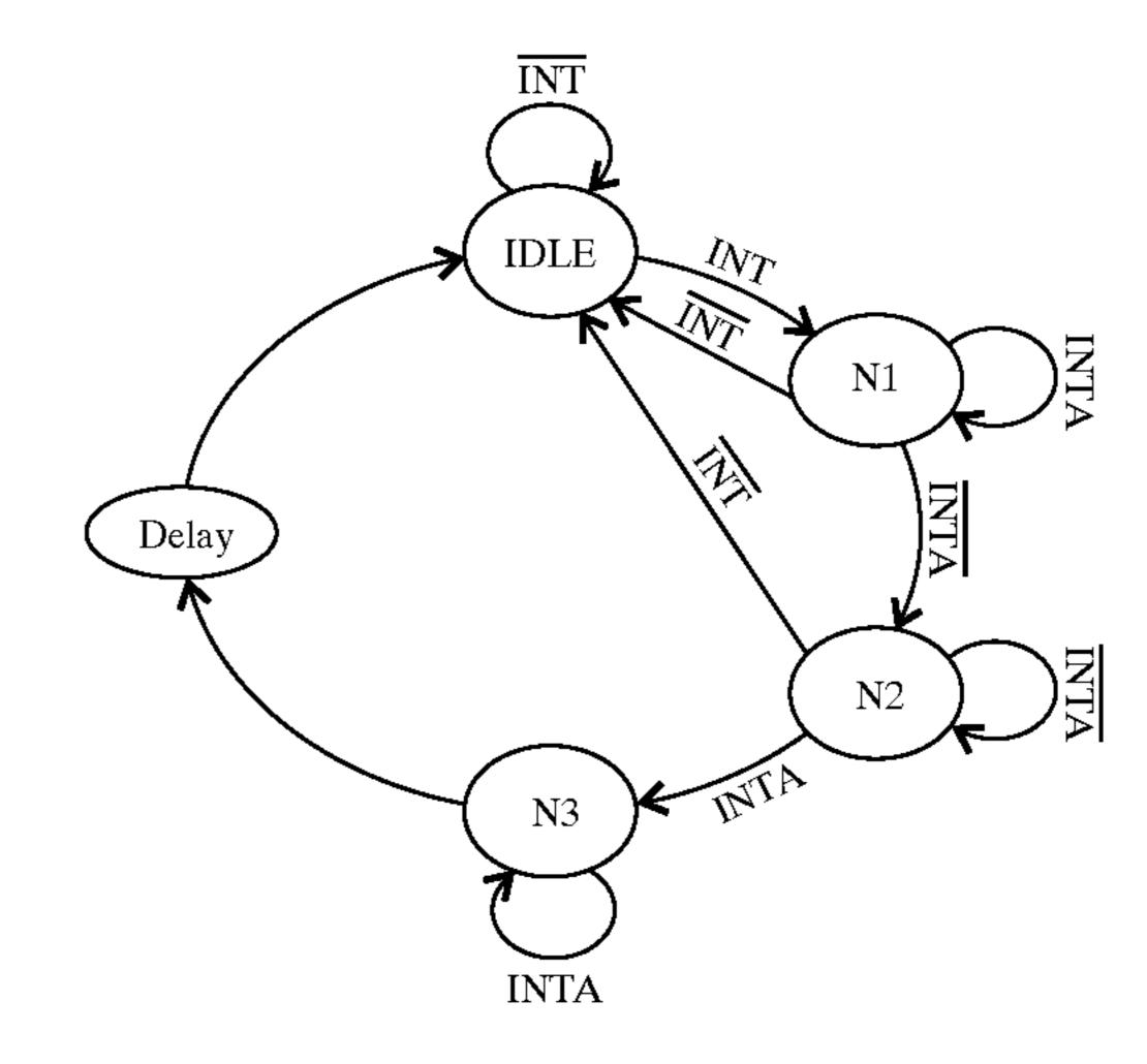
wherein when the state machine is in the N1, N2 and N3 states the state machine circuitry outputs an edge sensitive interrupt signal, when the state machine is in the Delay state the state machine circuitry outputs no interrupt signal, the INT signal comprising an active result of the logical OR operation of the interrupt lines from the first peripheral agents, the INTA signal comprising a signal from the CPU indicating that it is processing an interrupt.
