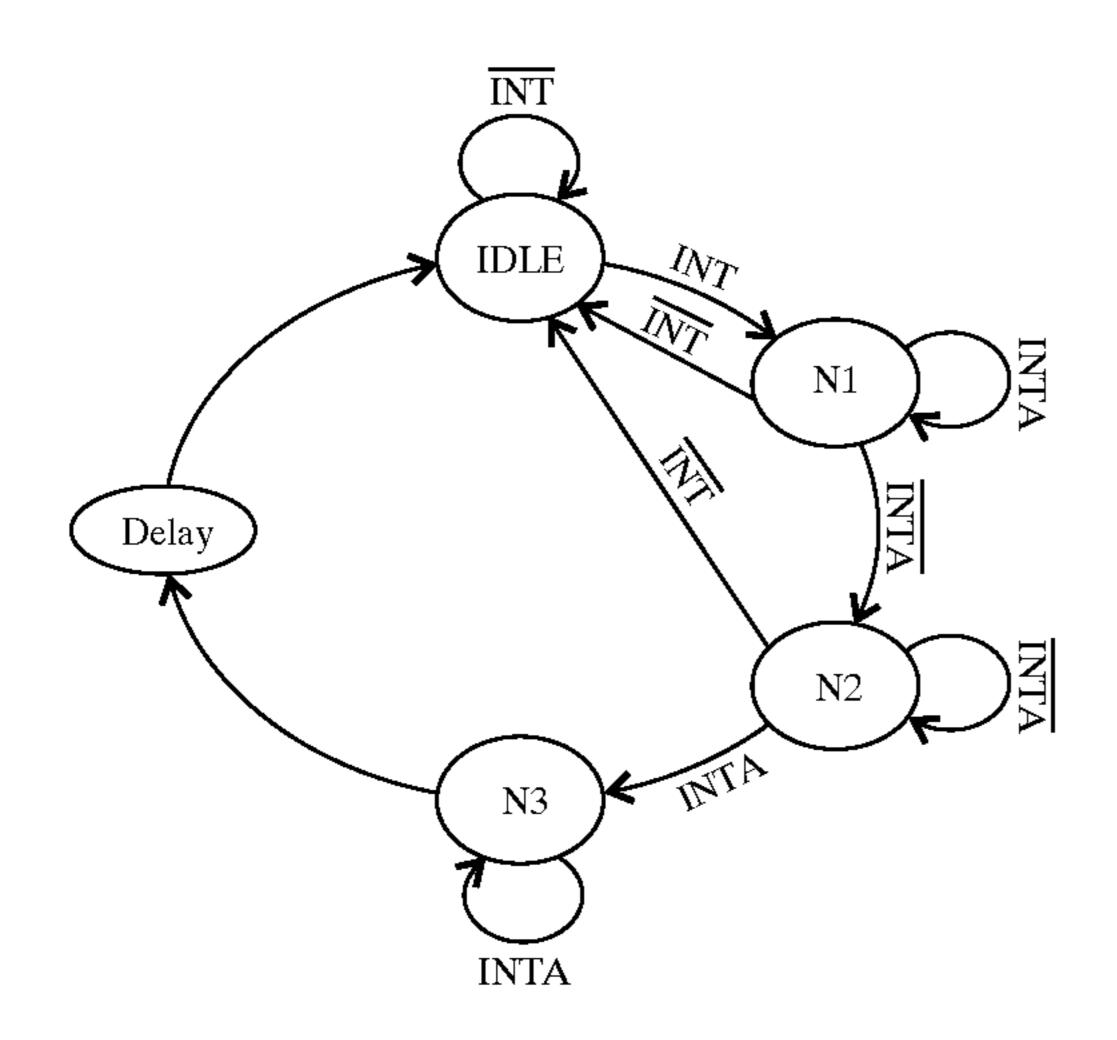
wherein when the state machine is in the N1, N2 and N3 states the state machine model outputs an edge sensitive interrupt signal to the interrupt controller, when the state machine is in the Delay state the state machine circuitry outputs no interrupt signal, the INT signal comprising an active result of the logical OR operation of the interrupt lines from the second peripheral agents, the INTA signal comprising a signal from the CPU indicating that it is processing an interrupt.
