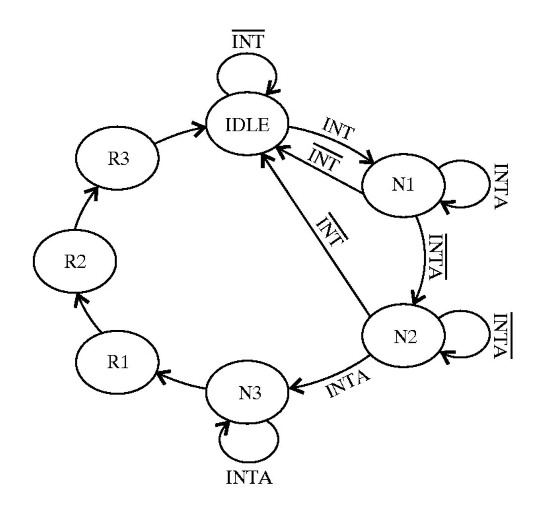
wherein when the state machine is in the N1, N2 and N3 states the state machine circuitry outputs an edge sensitive interrupt signal, the INT signal comprising an active result of the logical OR operation of the interrupt lines from the first peripheral agents, the INTA signal comprising a signal from the CPU indicating that it is processing an interrupt, the R1, R2 and R3 states comprising successive state machine states where the state machine circuitry outputs no interrupt signal.
