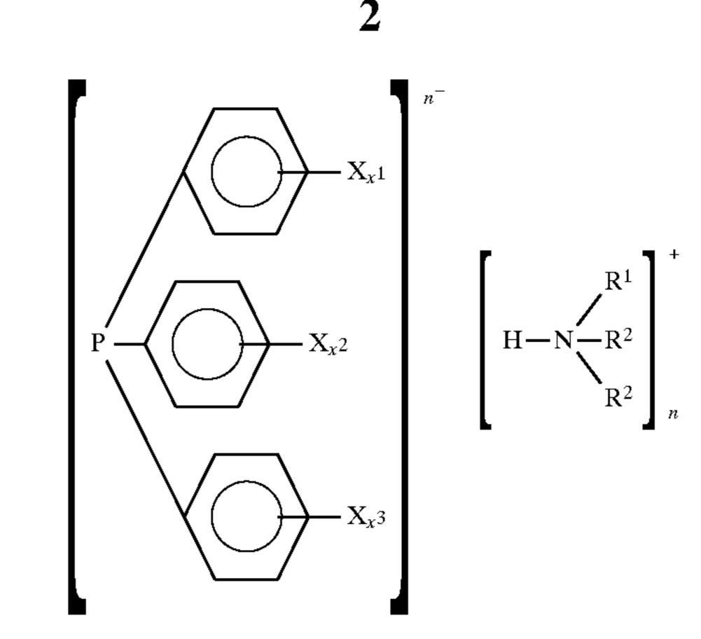
where X is sulfonate  $(SO_3^-)$  or carboxylate  $(COO^-)$ ,  $x^1$ ,  $x^2$  and  $x^3$  are 0 or 1,  $R^1$  and  $R^2$  are individually alkyl of 4 to 12 carbon atoms, aryl of 6 to 12 carbon atoms or cycloalkyl of 6 to 12 carbon atoms and  $R^1$  can additionally also be hydrogen.
