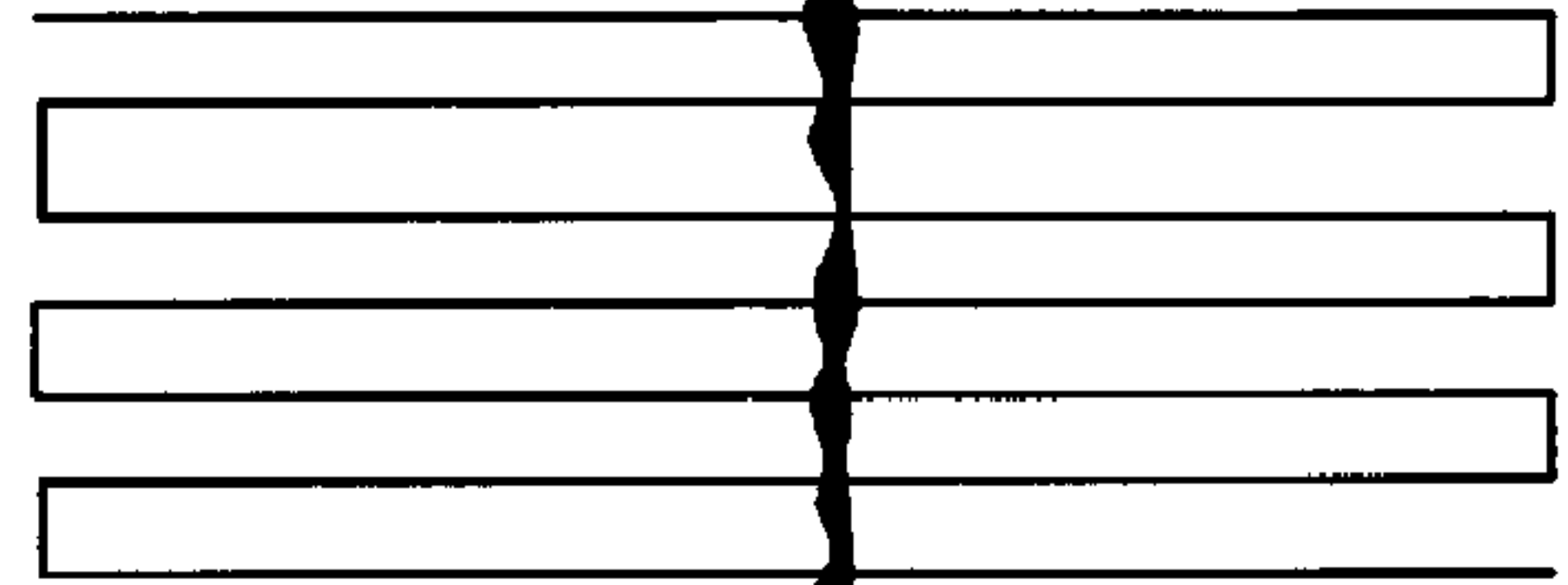
LOSS OF ADJACENCY IN VERTICAL DIRECTION
