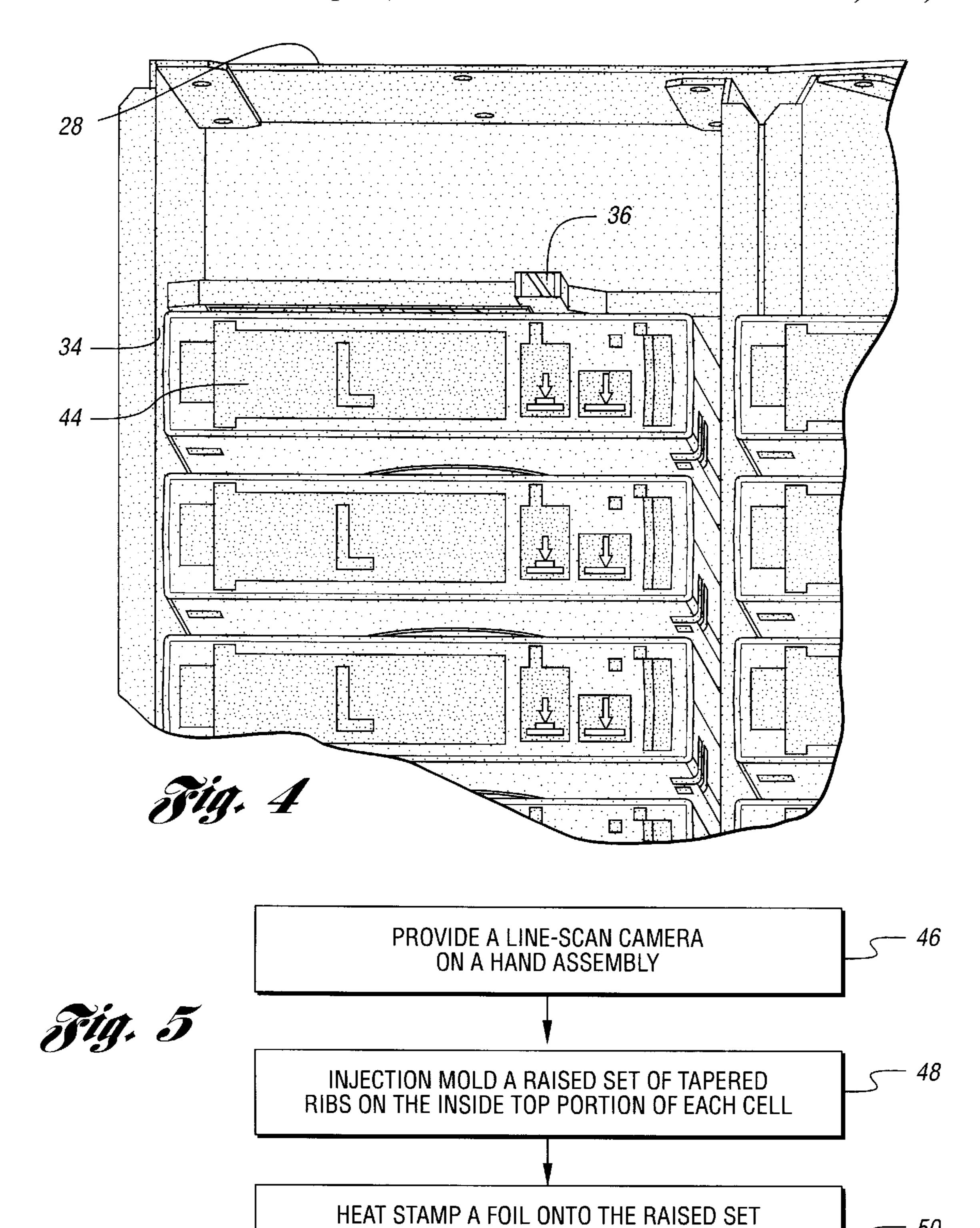
OPERATE THE LINE-SCAN CAMERA IN A MANNER TO SEARCH FOR THE VISIBLE PATTERN IN EACH CELL FOR AUDITING NUMBERS OF CARTRIDGES AND EMPTY CELLS IN THE STORAGE LIBRARY SYSTEM
