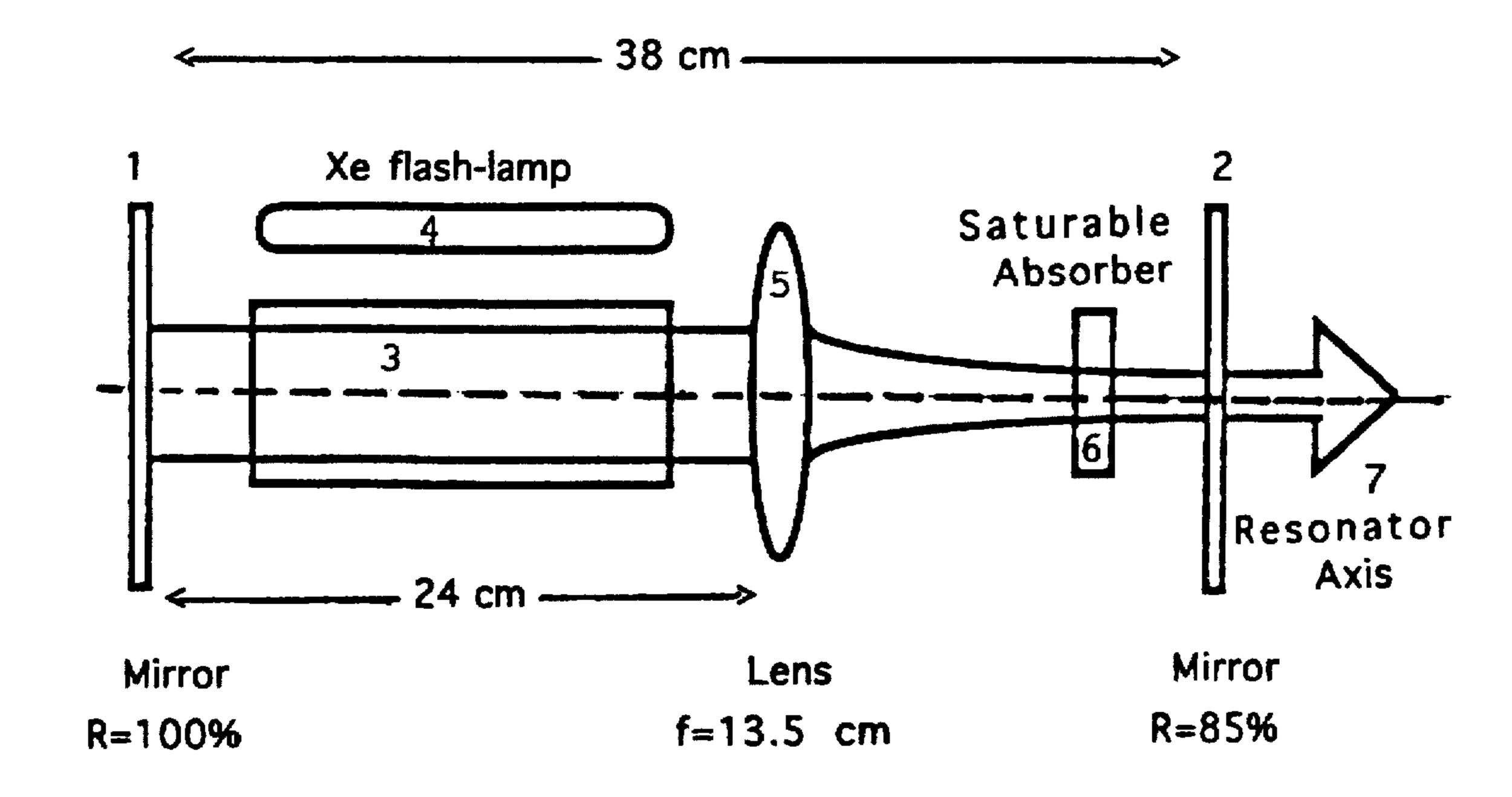
Fig. 1. Passive Q-switching experimental setup.
