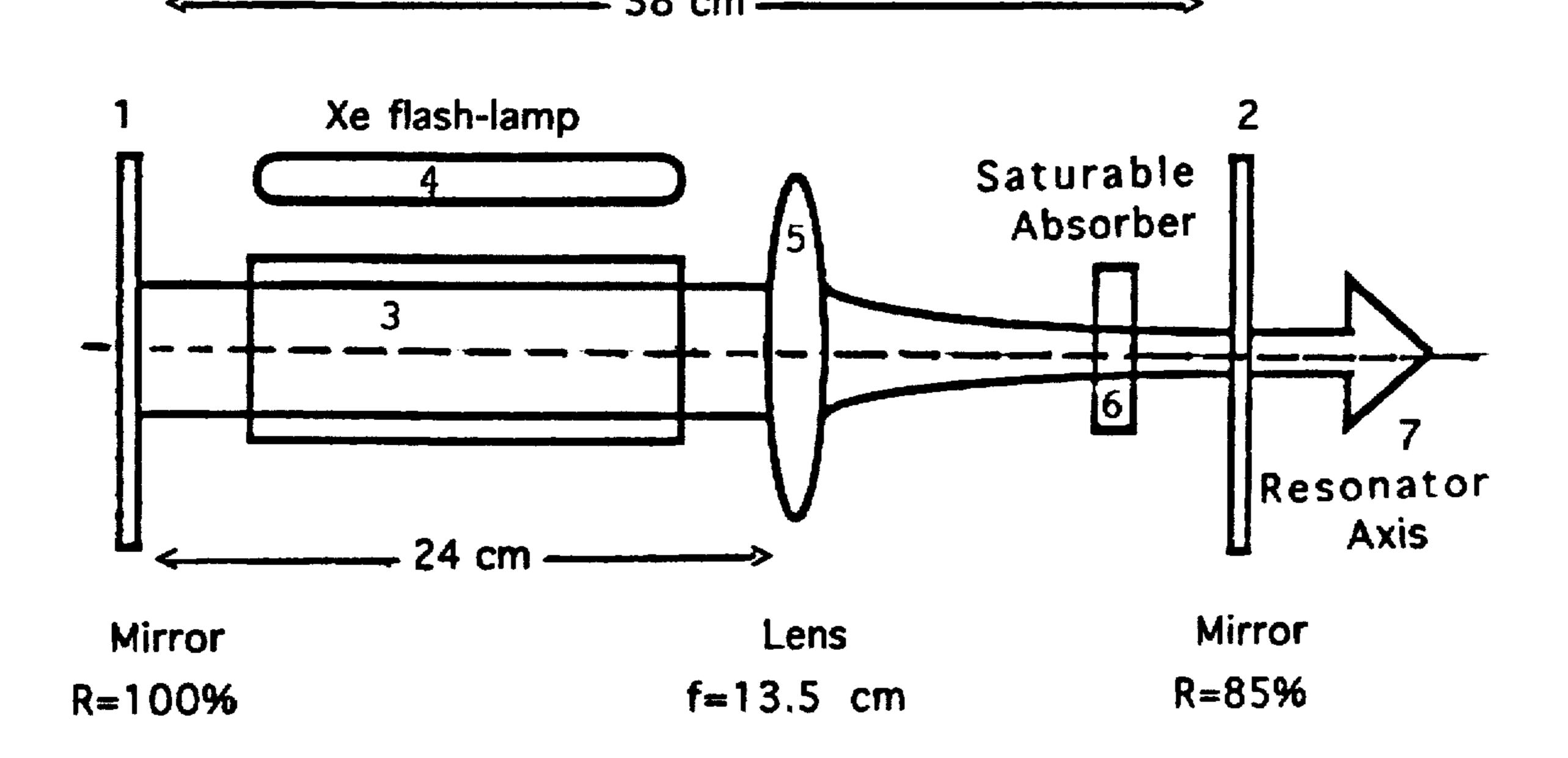
Passive Q-switching experimental setup.
