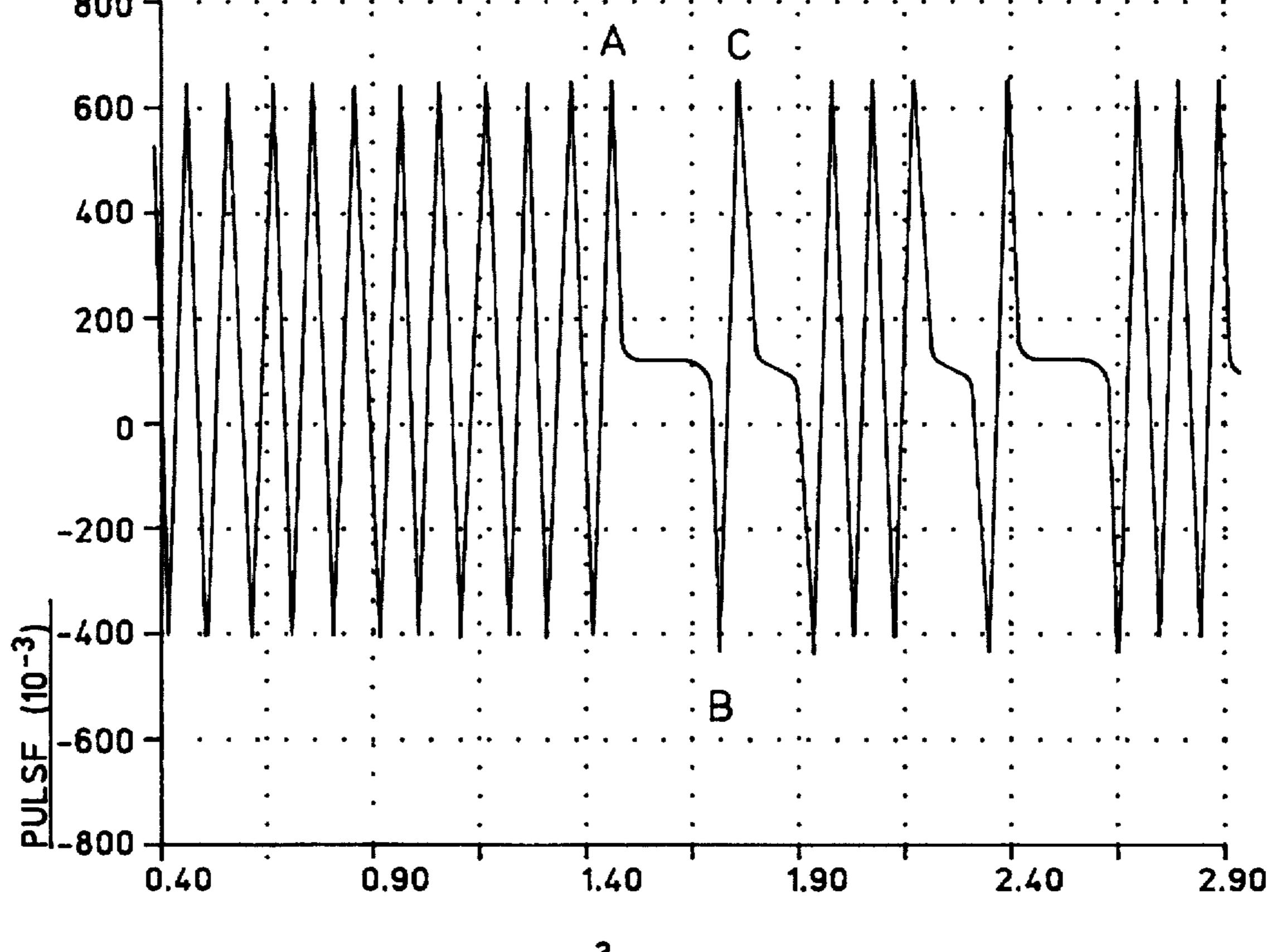
T (10<sup>3</sup> NANOSECONDS) 10 MHZ DIBIT PATTERN WITH NO ASYMMETRY OR AC COUPLING
