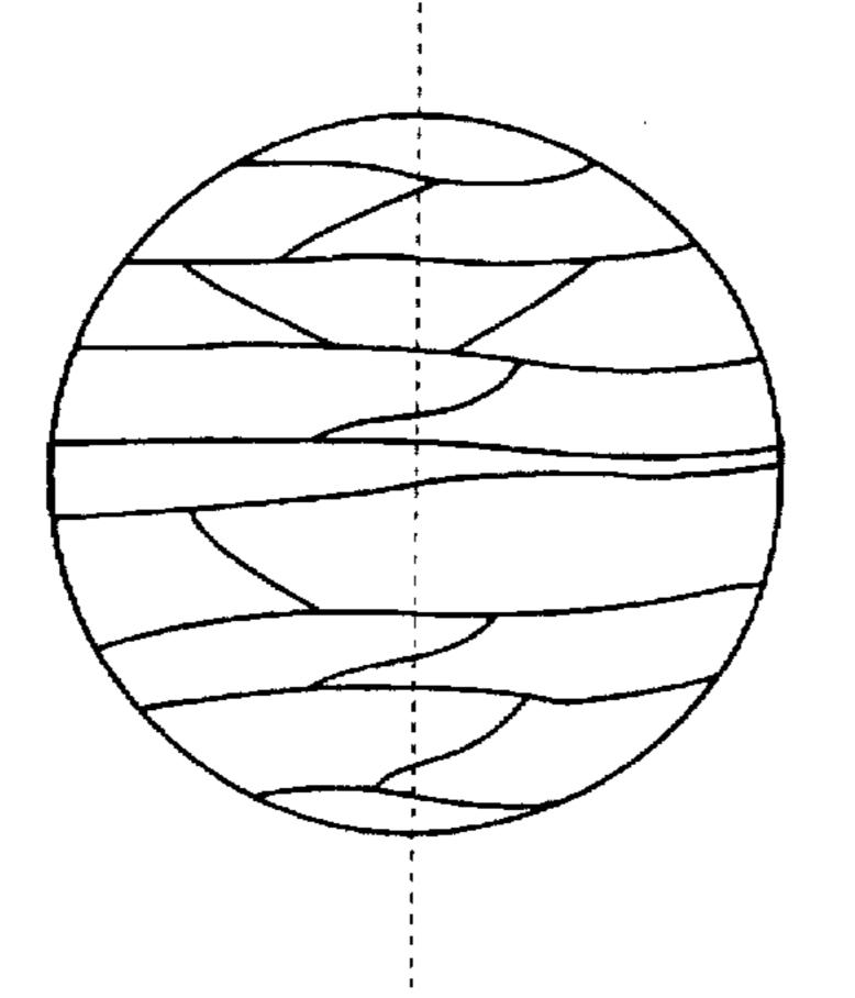
OLD AUSTENITE GRAIN BOUNDARY (INCLUSIVE OF DEFORMATION BAND AND TWIN CRYSTAL **BOUNDARY**)
