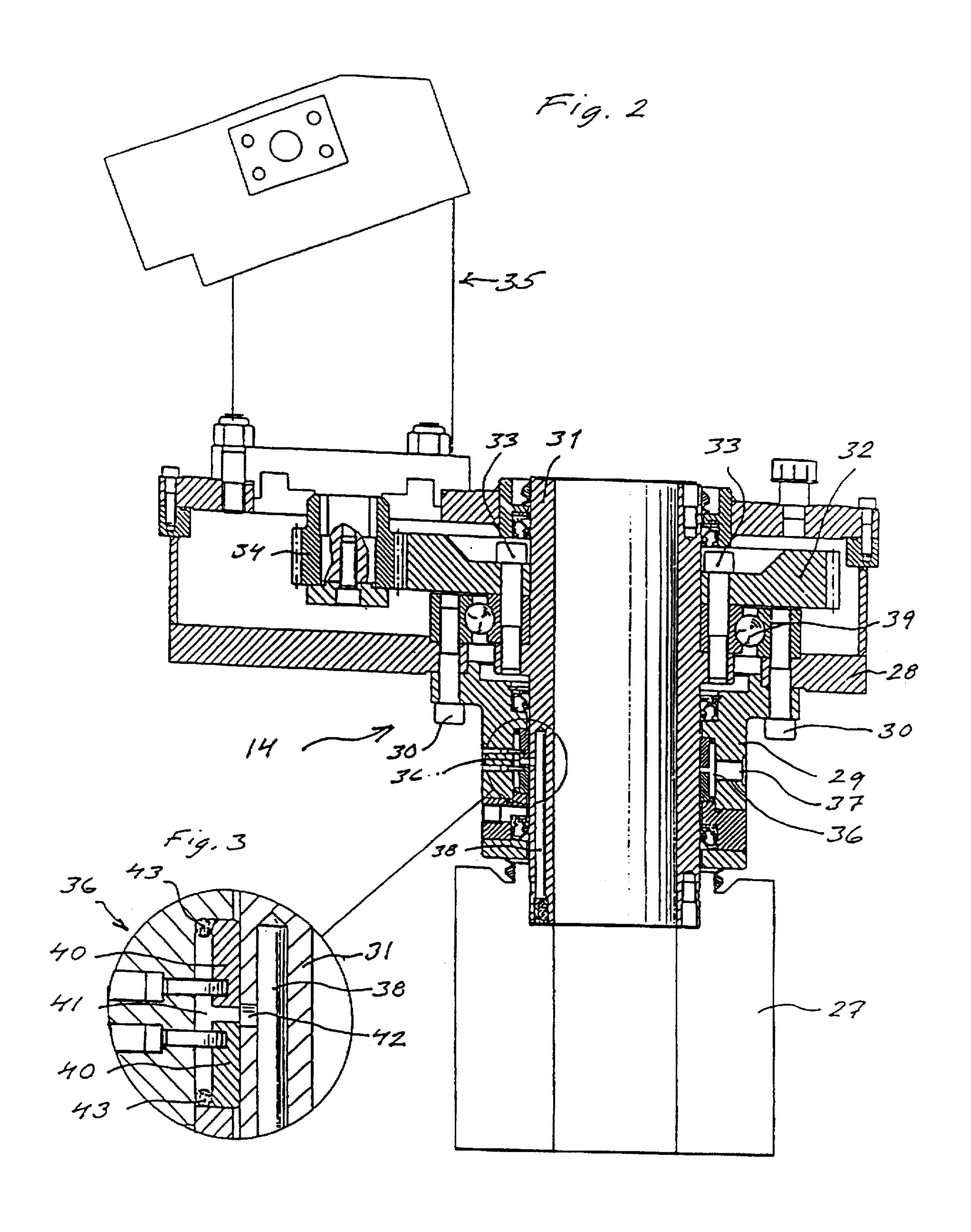
housing 14. This chuck accompanies the gear housing 14 as it moves axially.
