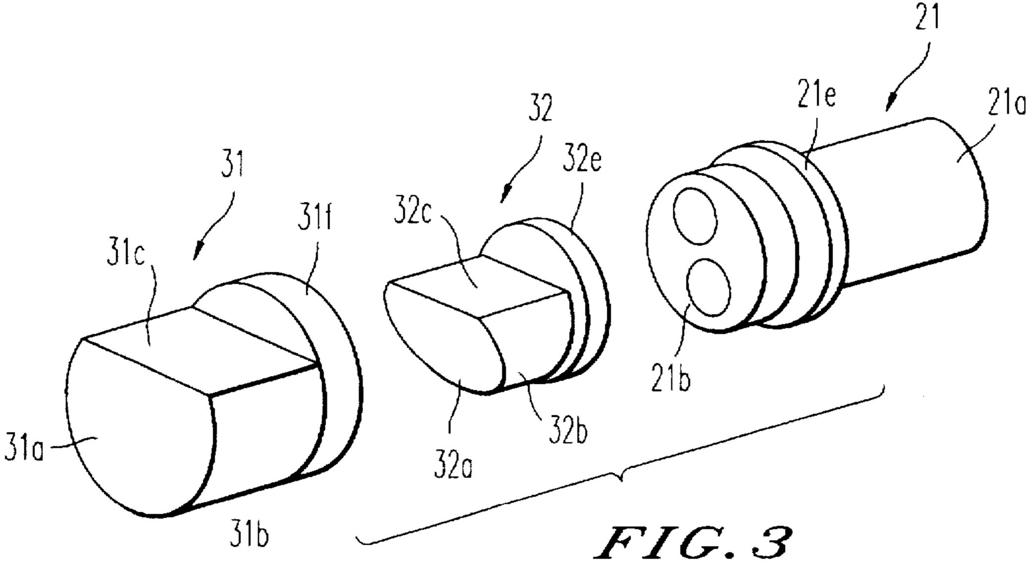
This invention relates to a photoelectric detector comprising an optical unit, in which are placed a transmitting optical component and a receiving optical component, which is fitted at the front with a front wall provided with lenses focused upon the optical axes of the beams transmitted and received by the components.
