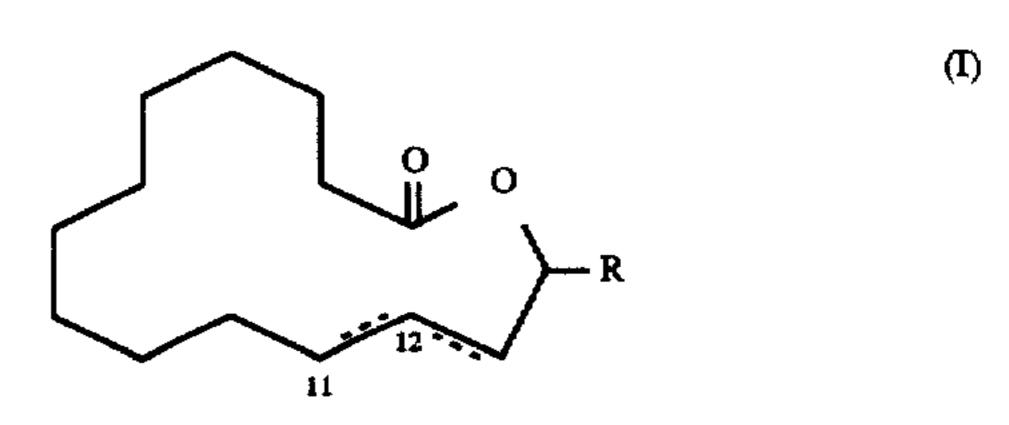
having a double bond in one of the positions indicated by the dotted lines and wherein symbol R represents a hydrogen atom or a methyl radical, which comprises the fragmentation of a hydroperoxide of formula
