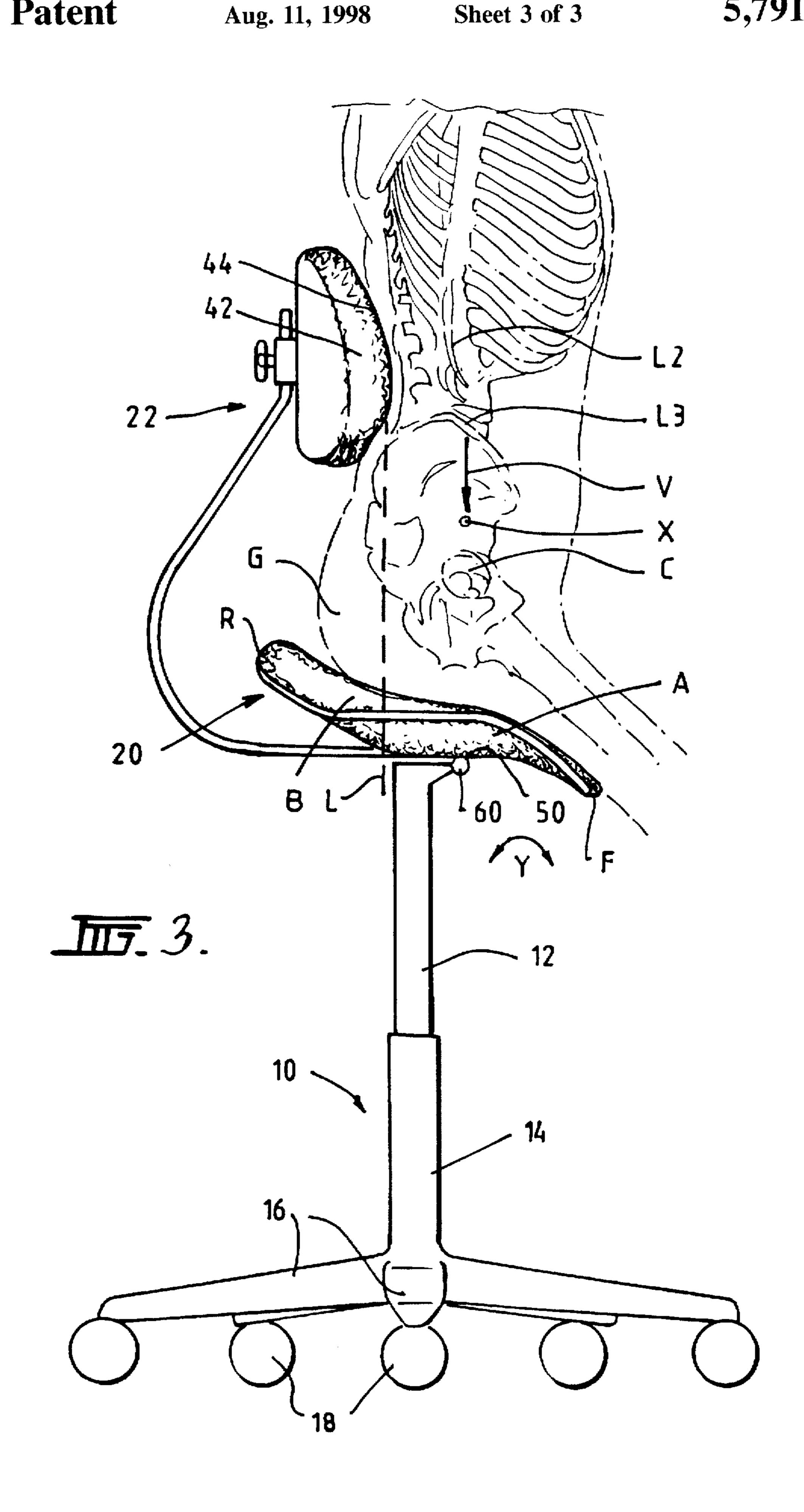
ERGONOMIC SEATING APPARATUS WITH INCLINED FEMORAL PORTION
