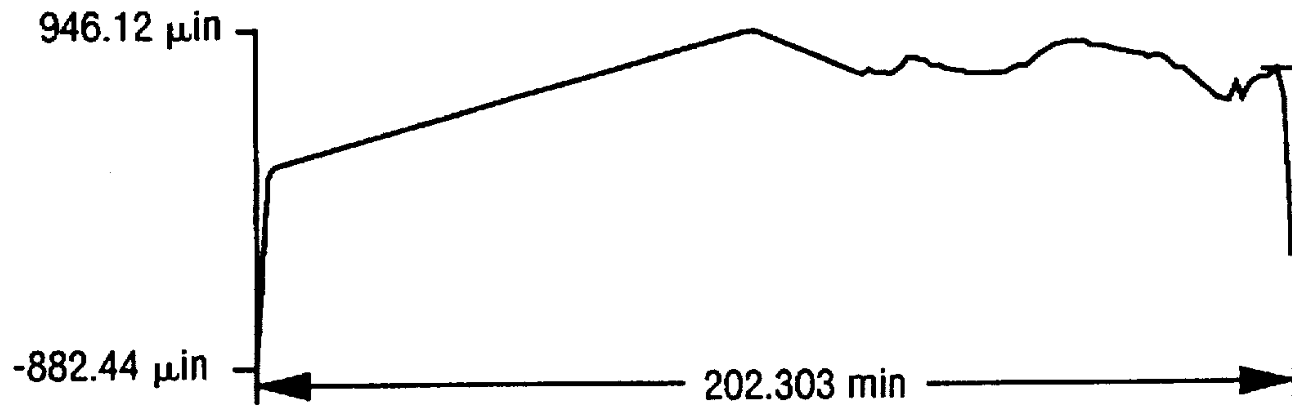
FIG. 8 Profile of the 440C head seal from Test #24.
