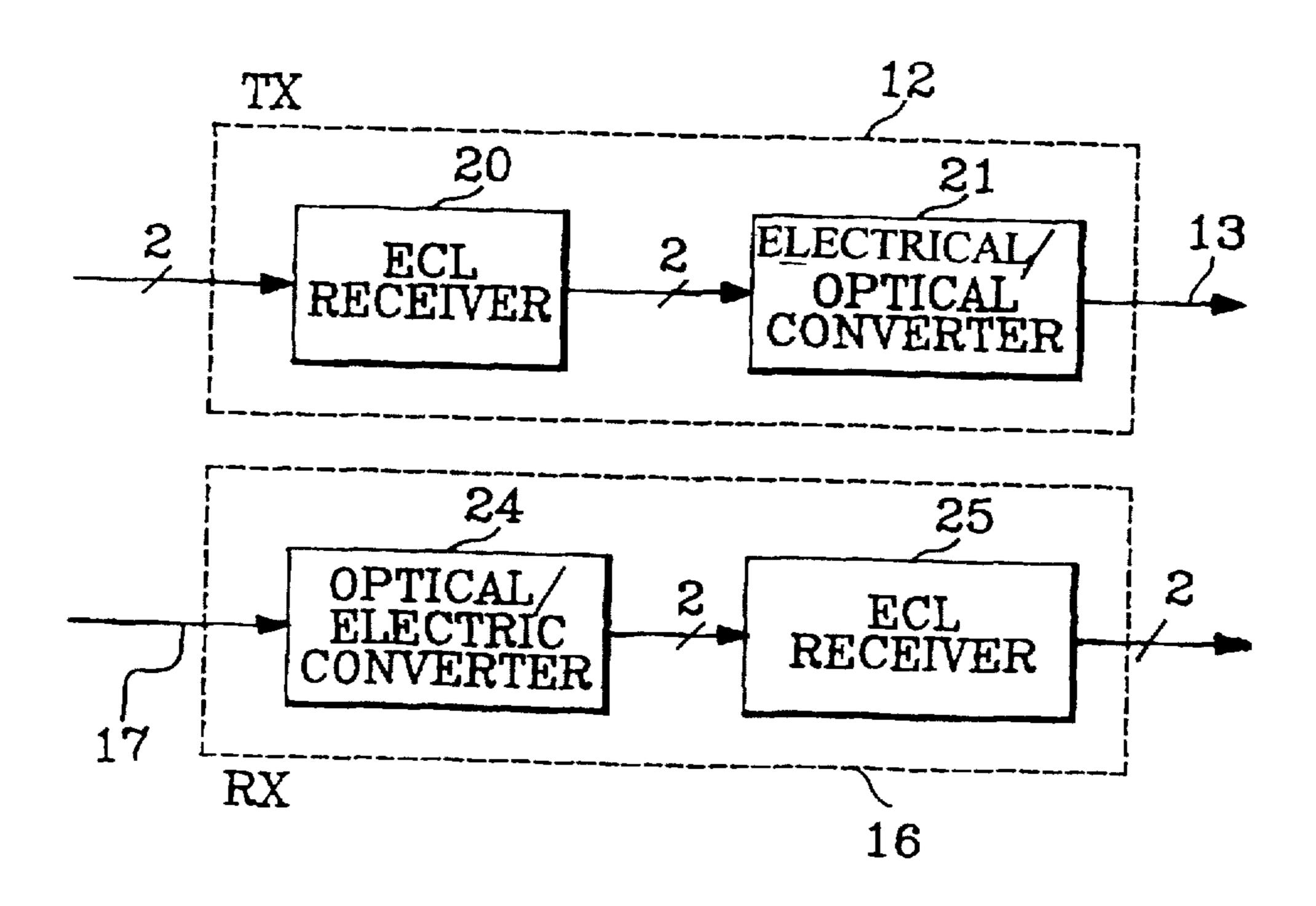
FIG. 2 Conventional Transceiver
