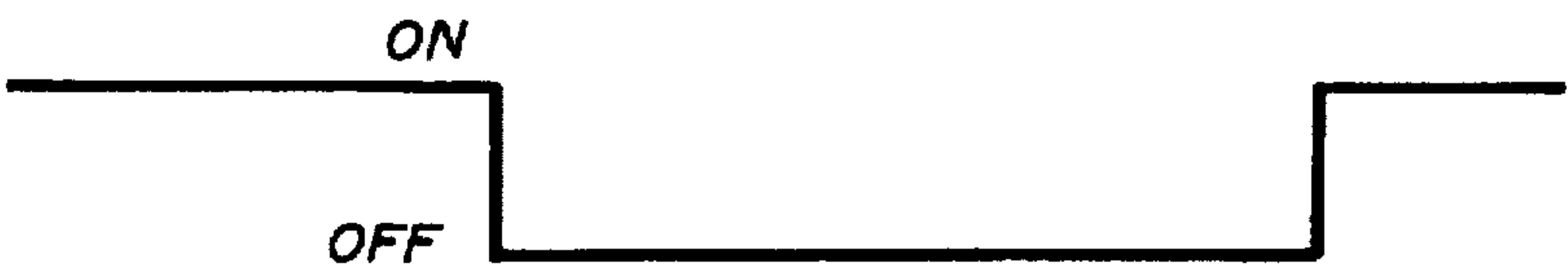
FIG.4C INPUT SIGNAL FOR E-LEVEL GATE
