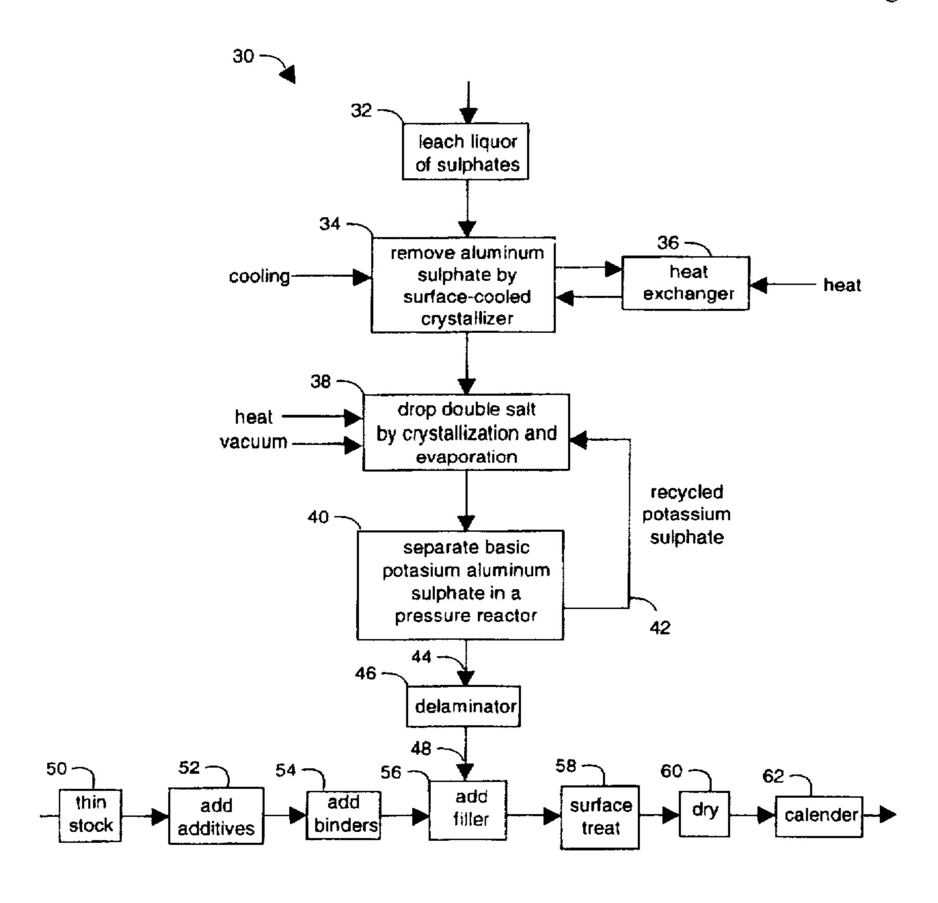
10 -12 -Fig. 1 leach liquor of sulphates 14 ~ 16 remove aluminum heat sulphate by cooling heat exchanger surface-cooled crystallizer 18 drop double salt heat by crystallization and vacuum ---evaporation recycled potassium 20 sulphate separate basic potasium aluminum sulphate in a pressure reactor 22 24 -26 delaminator 28 -BKAS
