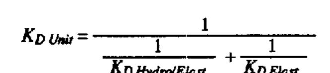
Where  $K_{D\ Unit}$  is the dynamic spring rate of the entire engine mount 10,  $K_{D\ Hydro/Elast}$  is the dynamic spring constant of the inner hydro-elastomeric spring 12, and  $K_{D\ Elast}$  is the dynamic spring constant of the outer elastomeric spring 14.
