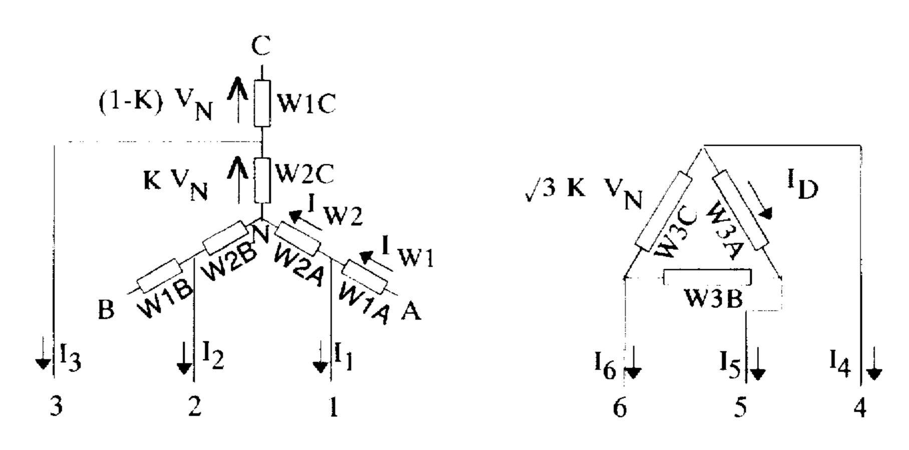
FOR K=0.5, TRANSFORMER VA = 0.58 DC LOAD W.
