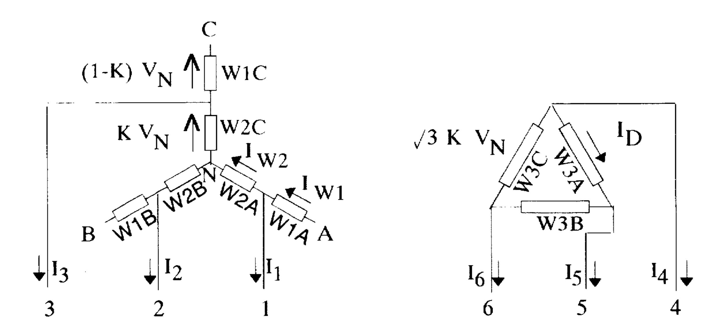
FOR K=0.5, TRANSFORMER VA = 0.58 DC LOAD W.
