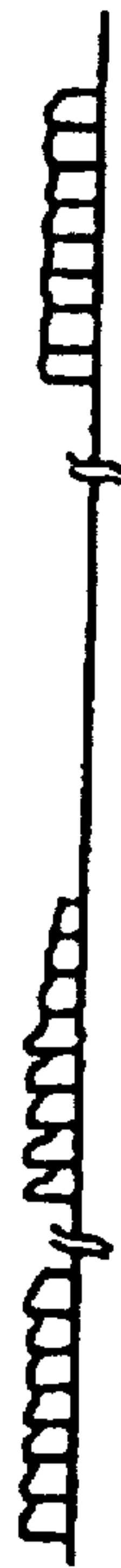
FIG. 9C OUTPUT IMAGE SIGNAL OF 2-ND OUTPUT PORT, DELAYED BY 1/2 V + a AND ENLARGED
