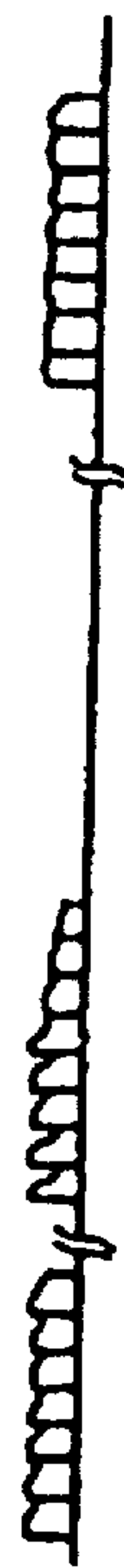
FIG. 9C OUTPUT IMAGE SIGNAL OF 2-ND OUTPUT PORT, DELAYED BY \frac{1}{2} V + a AND ENLARGED
