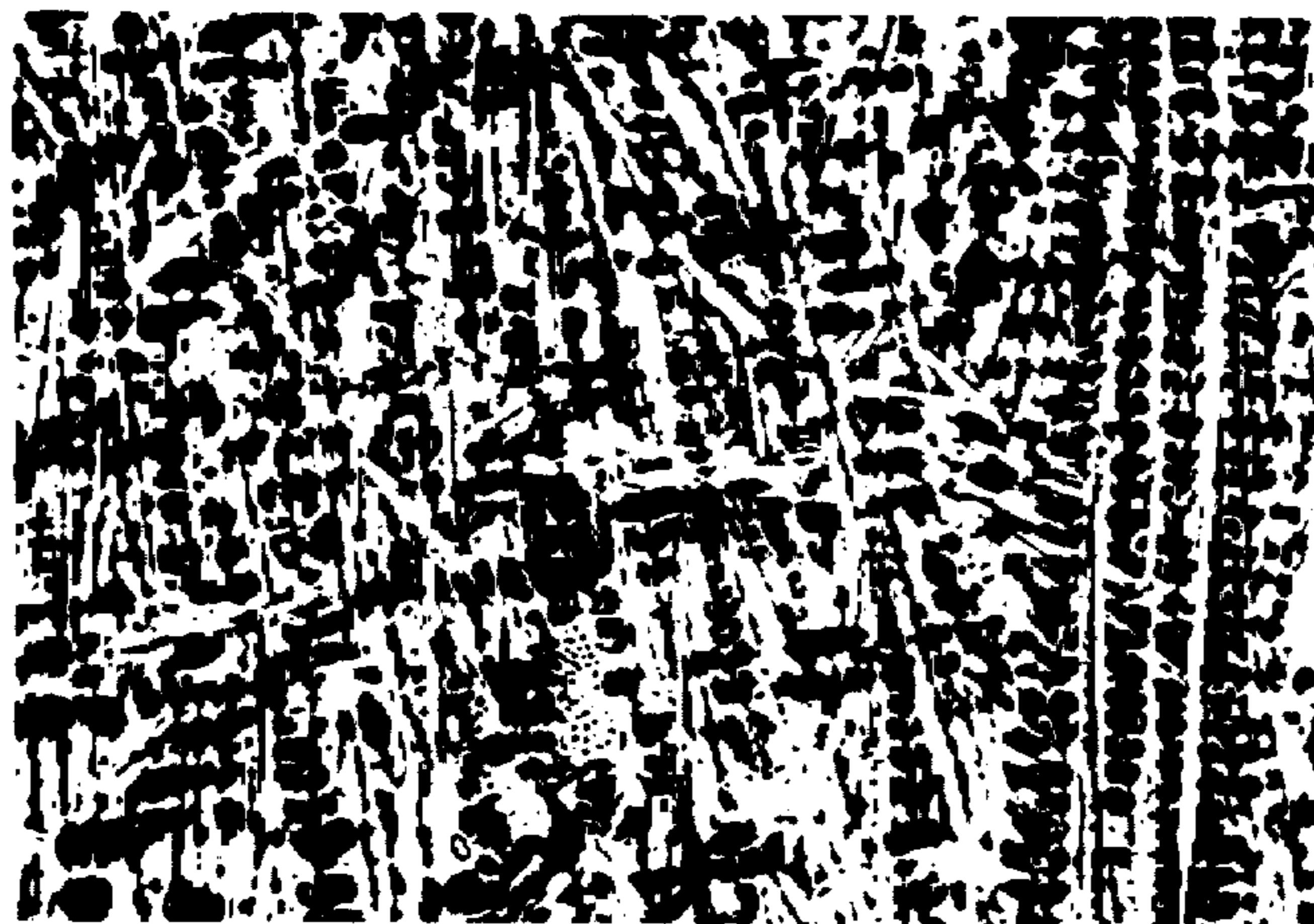
AVERAGE GRAIN DIAMETER 13 \mu\text{m}
