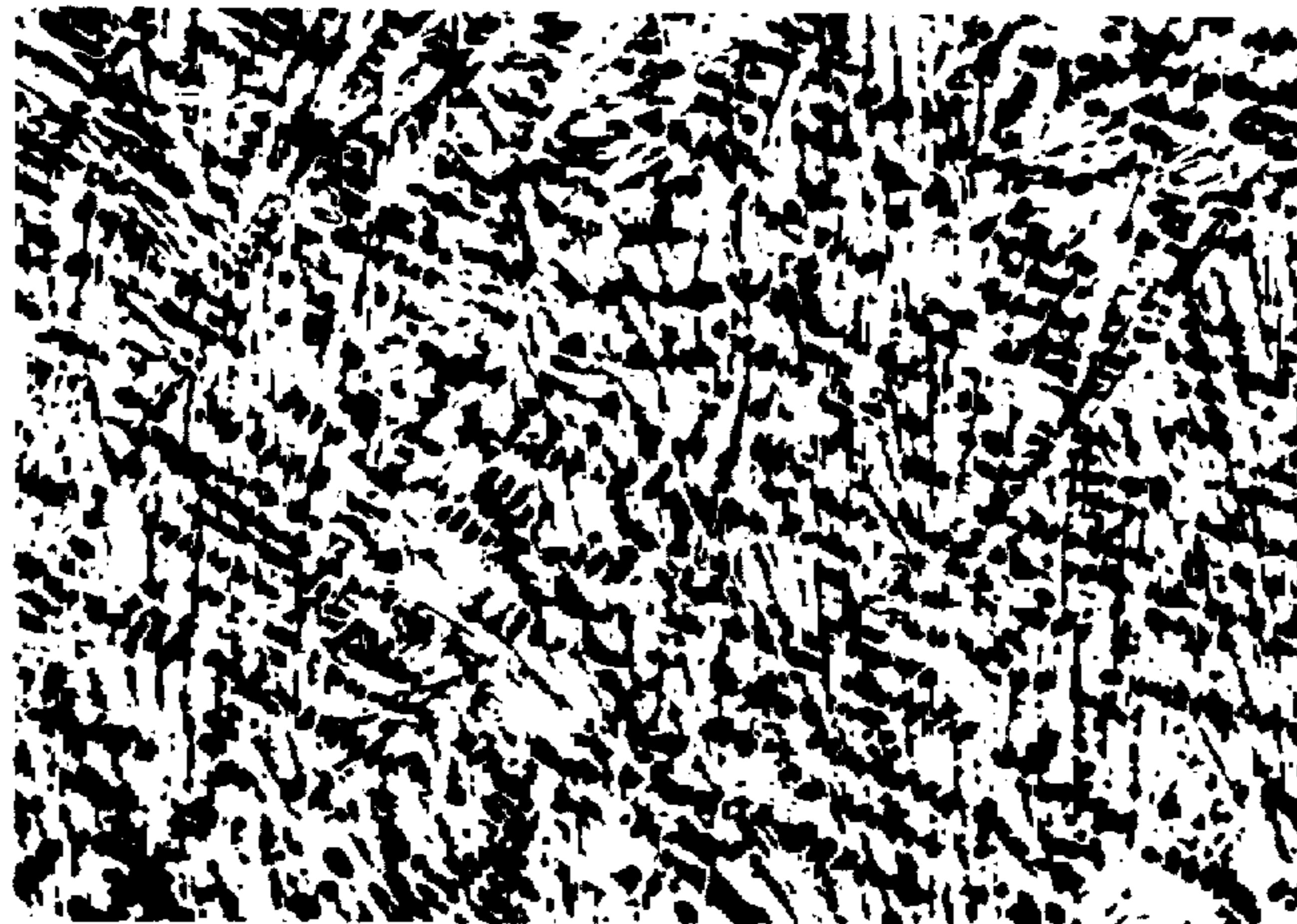
AVERAGE GRAIN DIAMETER 8 \mu\text{m}
