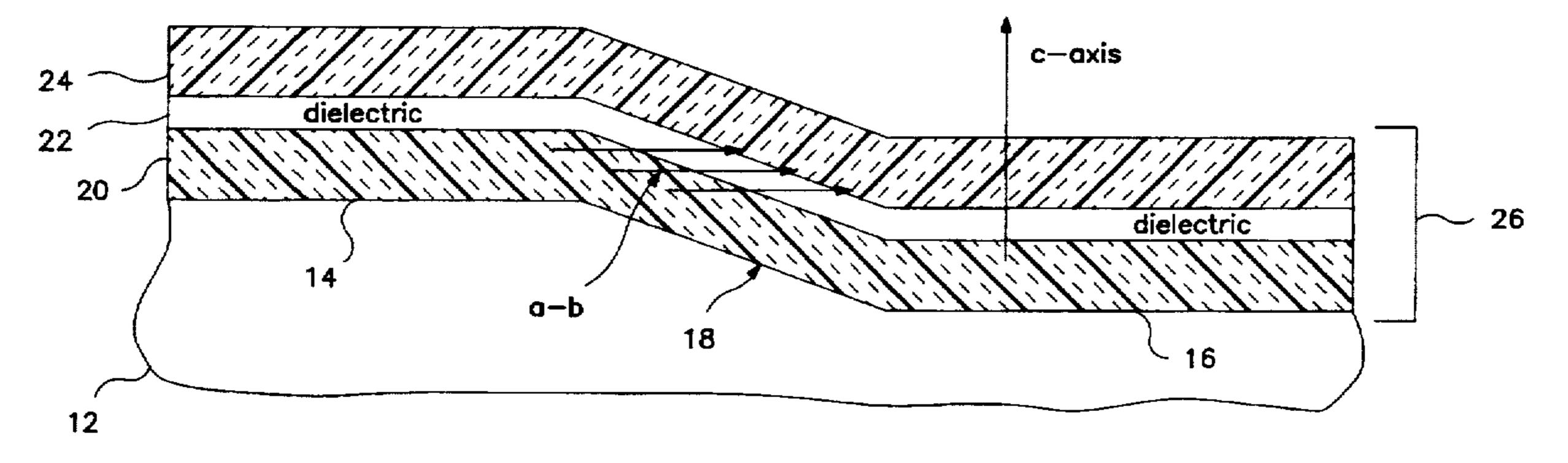
etching a planar substrate to yield a first planar segment, a second planar segment, and a ramp segment, the ramp segment connecting the two planar segments at an angle thereto, the substrate being thinner in the second planar segment than in the first planar segment, and the substrate having a constantly—decreasing thickness in the ramp segment
