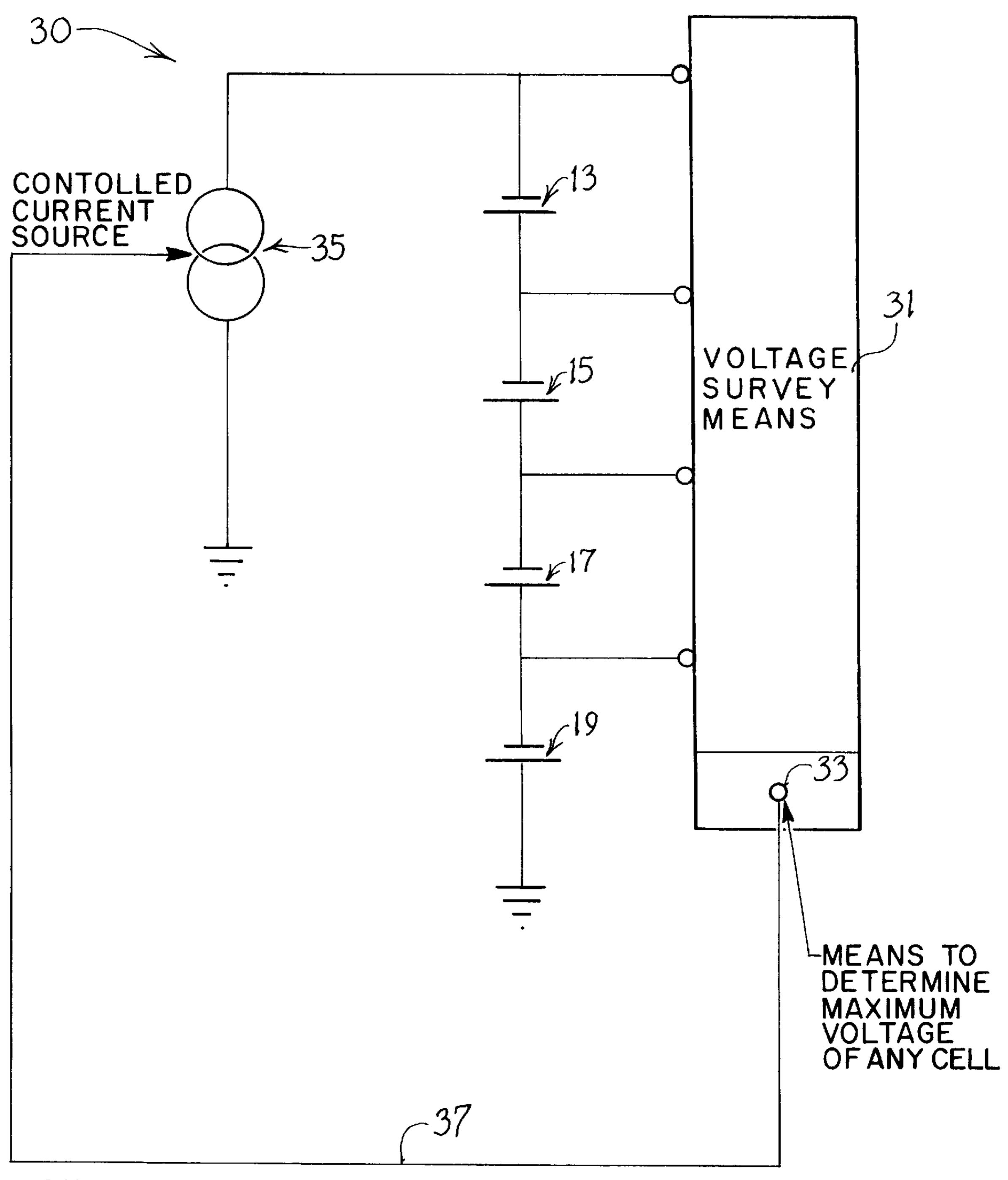
SET CURRENT TO LIMIT MAXIMUM VOLTAGE OF HIGHEST VOLTAGE CELL
