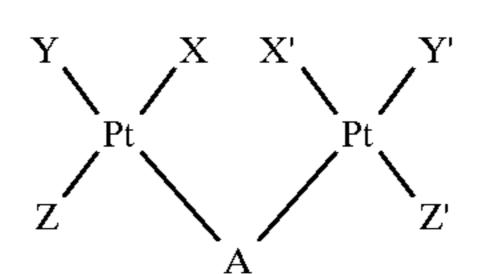
wherein X, Y, Z, X', Y', and Z' are the same or different ligands and are halide, sulphate, phosphate, nitrate, carboxylate, substituted carboxylate, dicarboxylate, substituted dicarboxylate primary or secondary amine, sulfoxide, phosphine, pyridine-type nitrogen and the like; preferably, there is at least one Pt-anion bond on each Pt molecule; and A is a diamine or polyamine.
