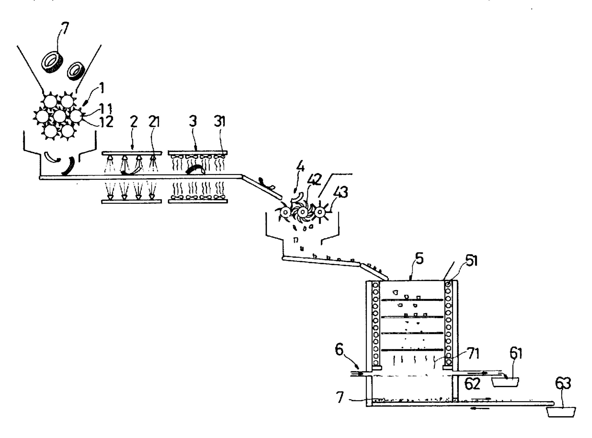
First step: using a grinding device to grind the waste tire into blocks or cubes with smaller volume
