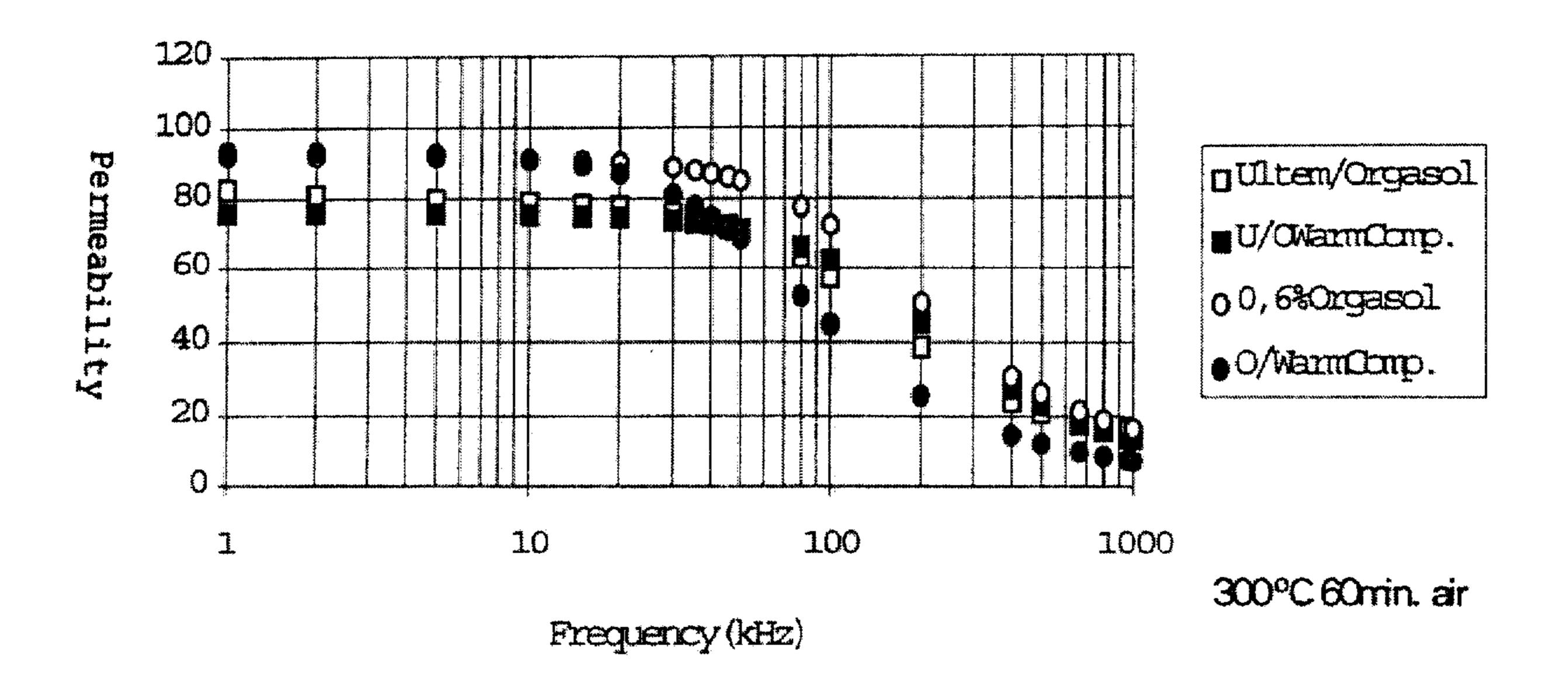
FIG.4 ABM100.32 with Ultern D.M. + Orgasol & 0,6% Orgasol both Warm & Cold Compacted Compared to the Referance containing 0,5% Kenolube
