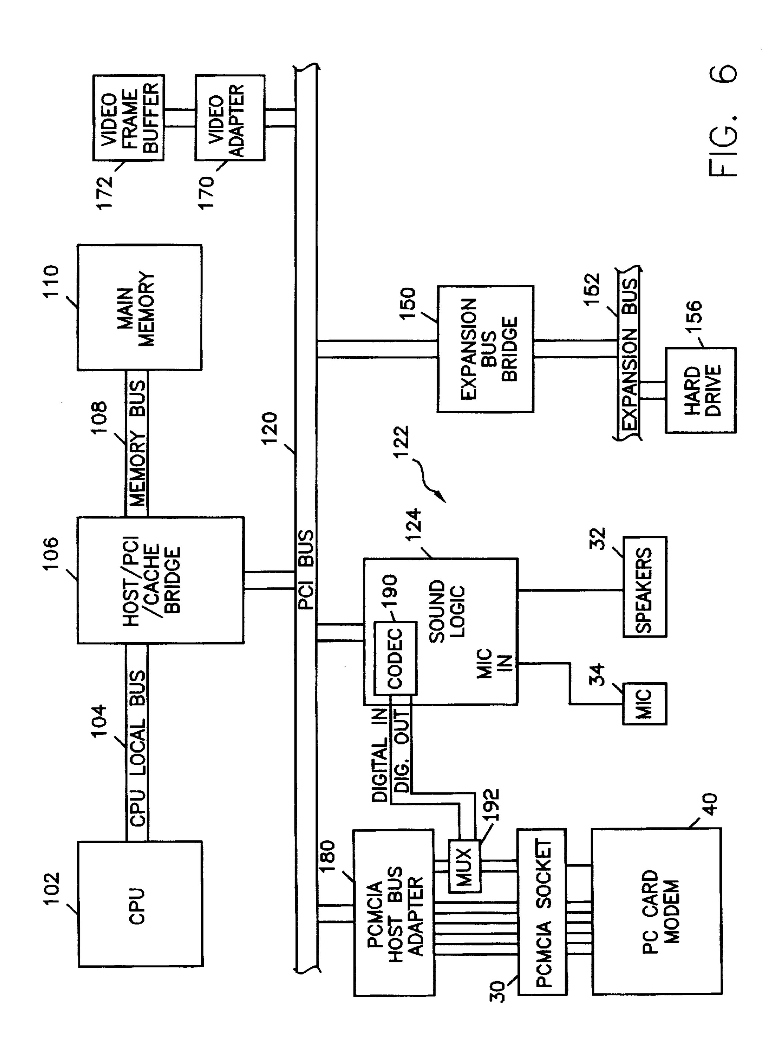
SYSTEM FOR MULTIPLEXING PINS OF A PC CARD SOCKET AND PC CARD BUS ADAPTER FOR PROVIDING AUDIO COMMUNICATION BETWEEN PC CARD AND COMPUTER SOUND SYSTEM
