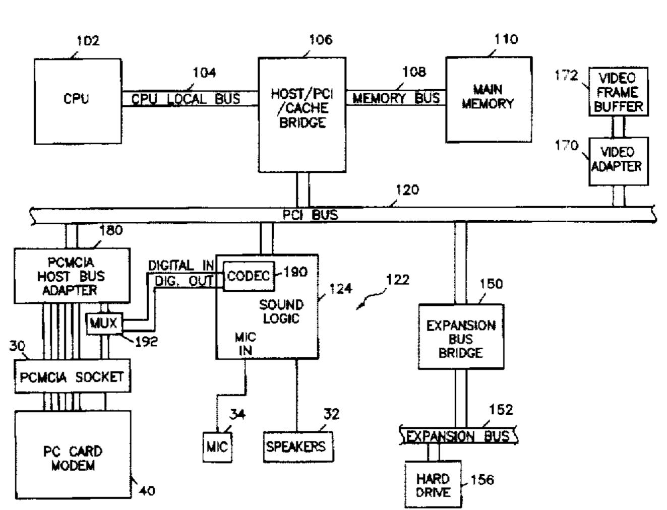
digital audio signals between the PC Card and the computer sound system.
