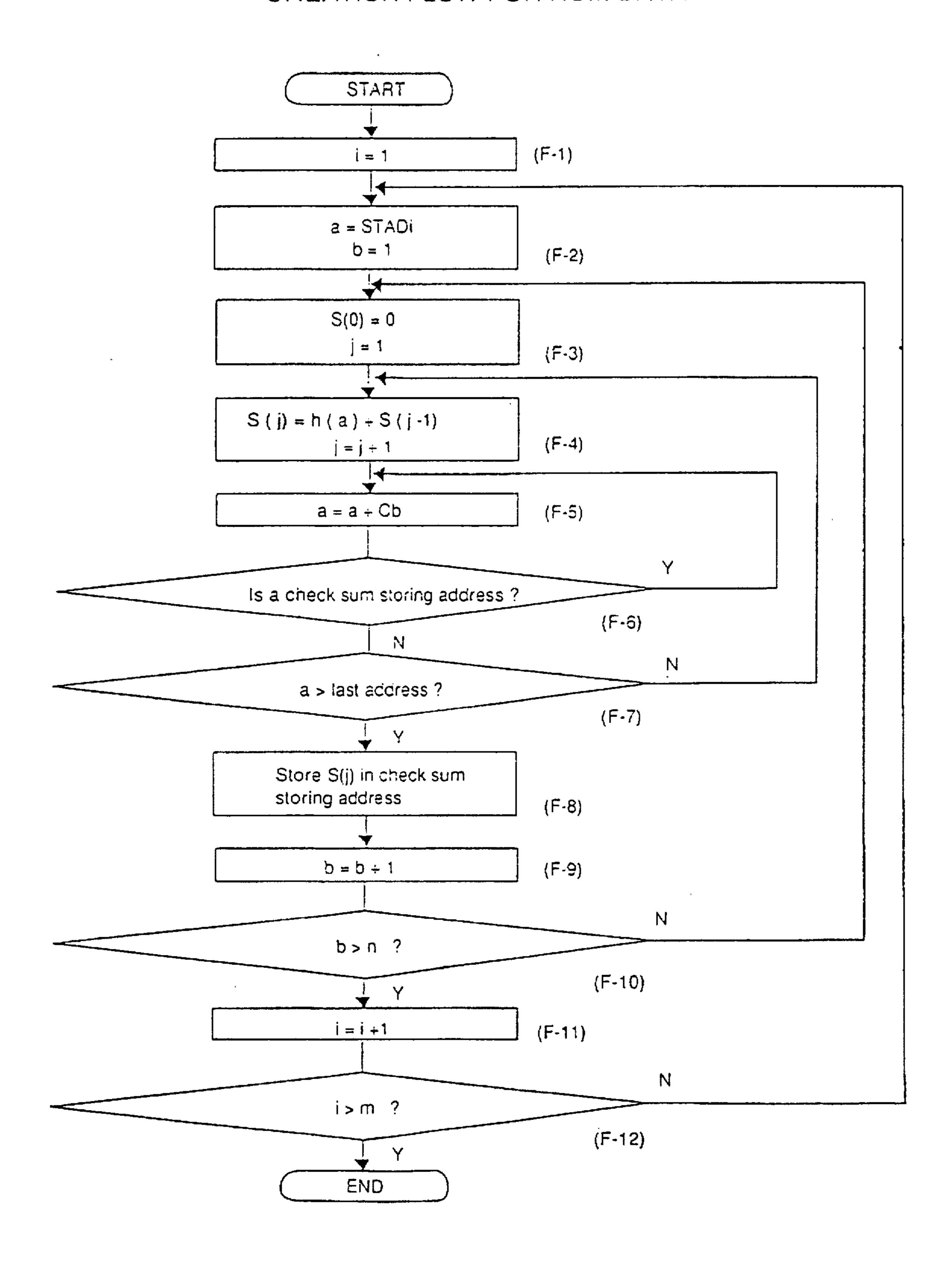
FIG.4 CHECK FLOW FOR EXTERNAL ROM
