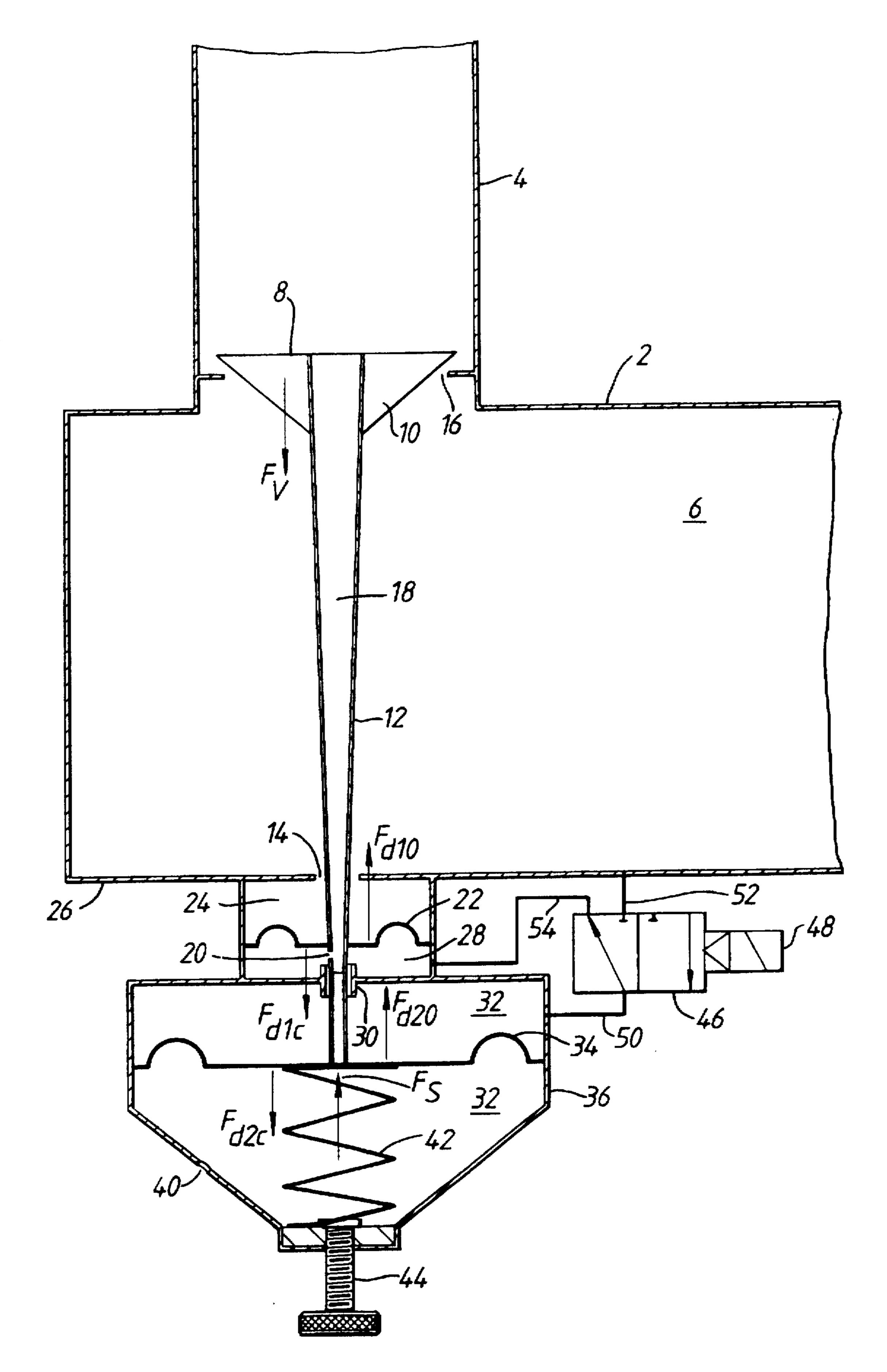
The present invention relates to meters and in particular to a gas meter having a governor which is used to control the flow of gas through the meter.
