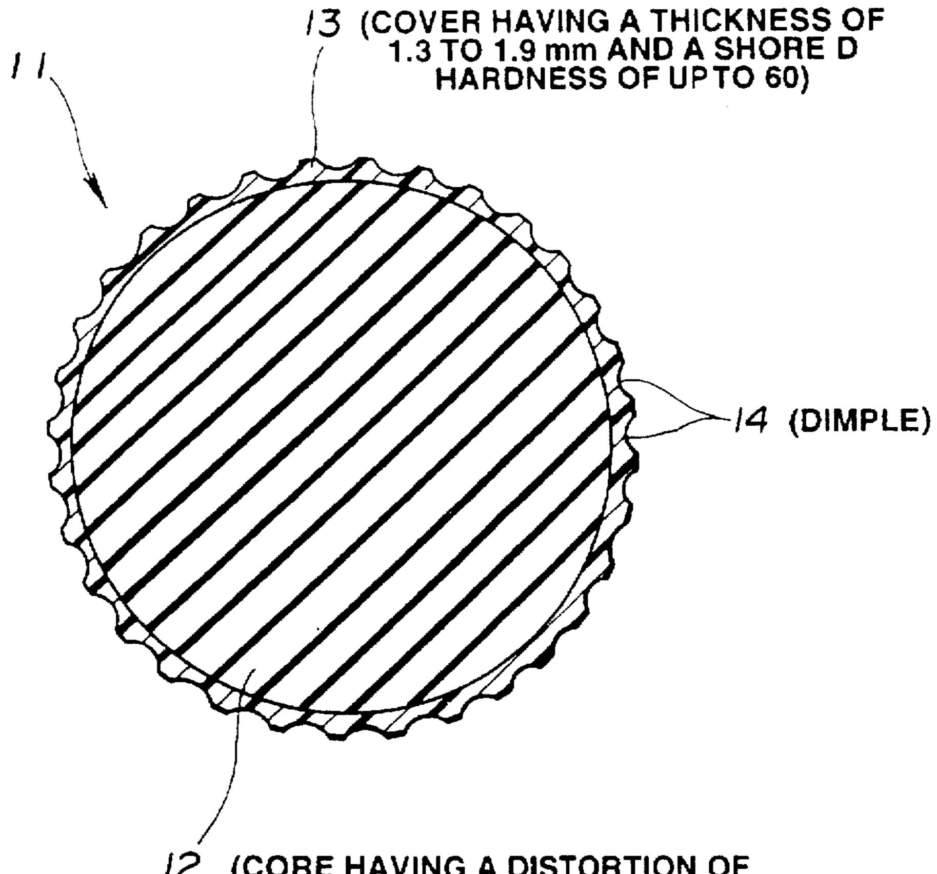
12 (CORE HAVING A DISTORTION OF 2.9 TO 4.0 mm UNDER A LOAD OF 100kg AND RATIO OF CORE DISTORTION/BALL DISTORTION OF 1.0 TO 1.3)
