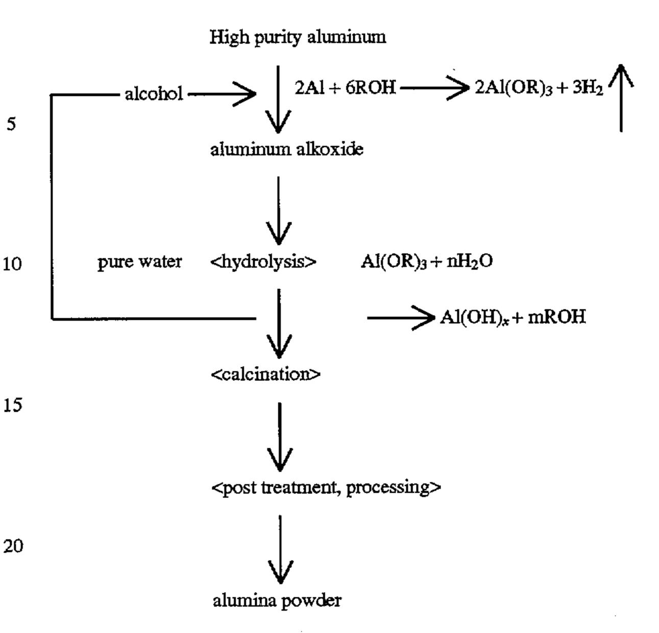
In the above process, metallic aluminum is reacted with an alcohol, such as methanol, to form an alkoxide, which is then hydrolyzed to provide aluminum hydroxide. The aluminum hydroxide is then calcined to obtain powdery alumina.
