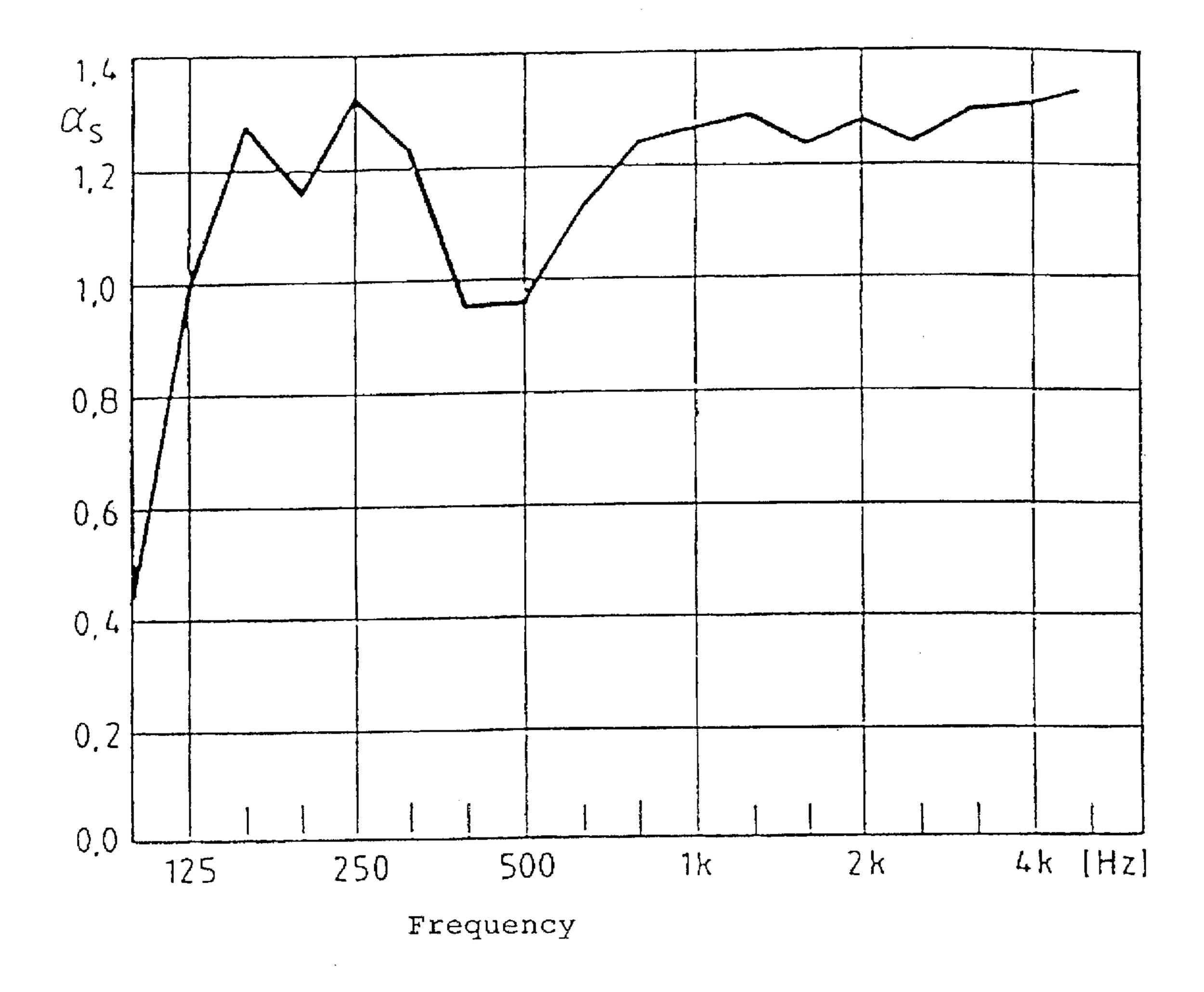
Fig. 4 Degree of absorption of membrane absorbers according to fig. 3 (but without a covering membrane) having a 50mm thick mineral wool layer.
