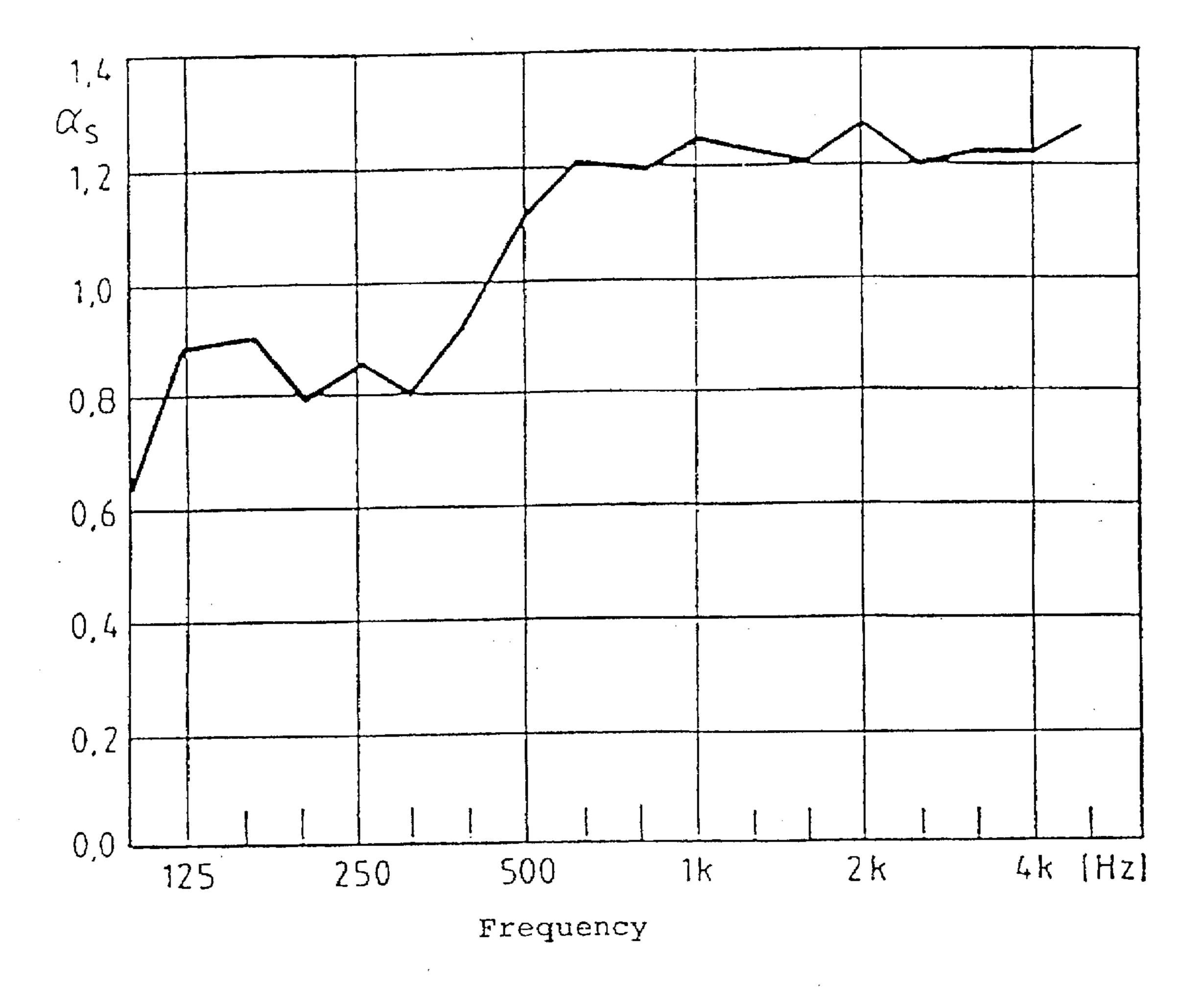
Fig. 5 Degree of absorption of membrane absorbers according to fig. 3 having a 50 mm thick mineral wool layer.
