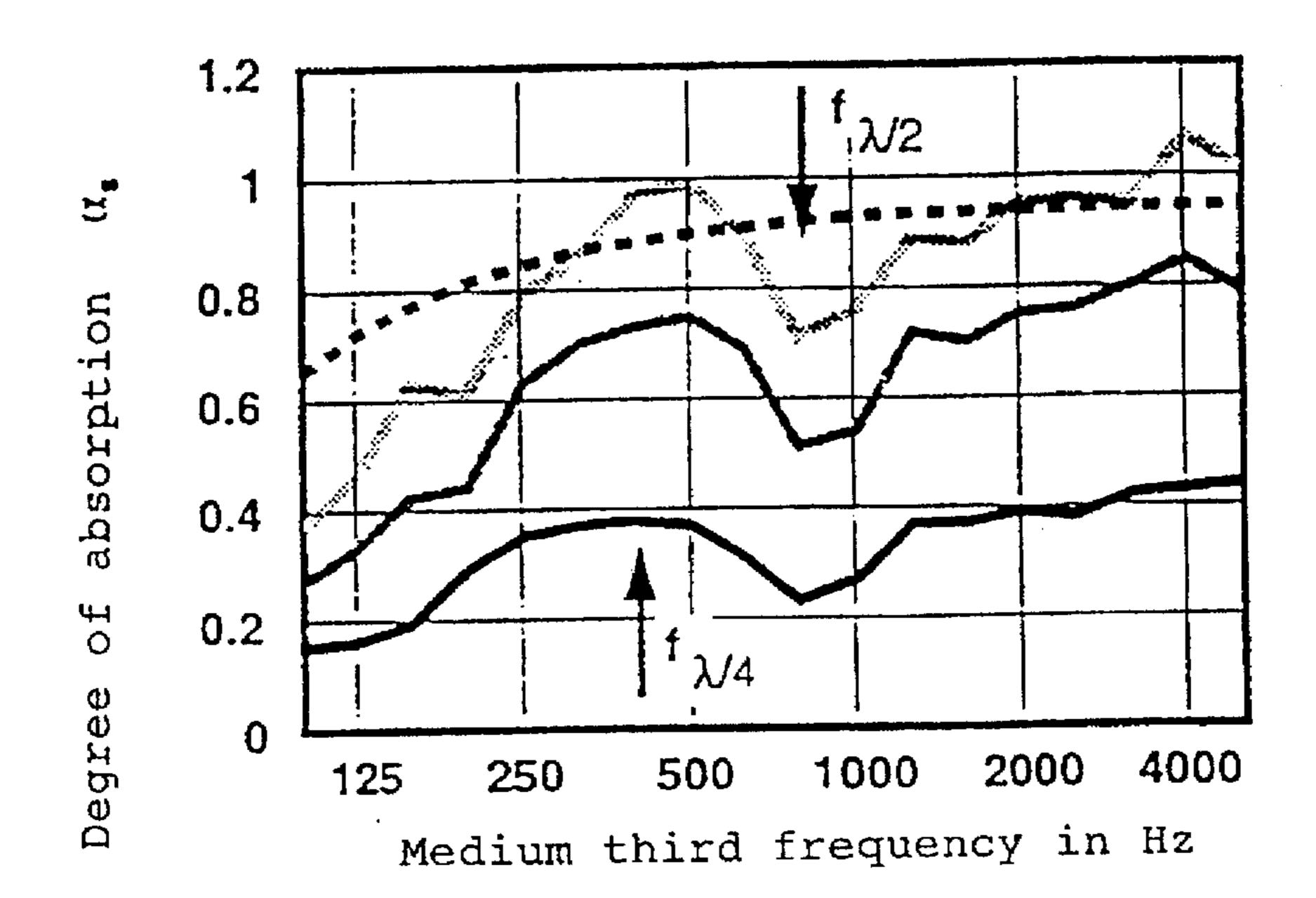
Vlies Typ A, 0.6 mm Vlies Typ A, 5.0 mm, 500 g/m<sup>2</sup> Vlies Typ A, 7.0 mm, 1000 g/m<sup>2</sup> Homogeneous porous  $\Xi = 8 \text{ kNs/m}^4$ , 200 mm absorber
