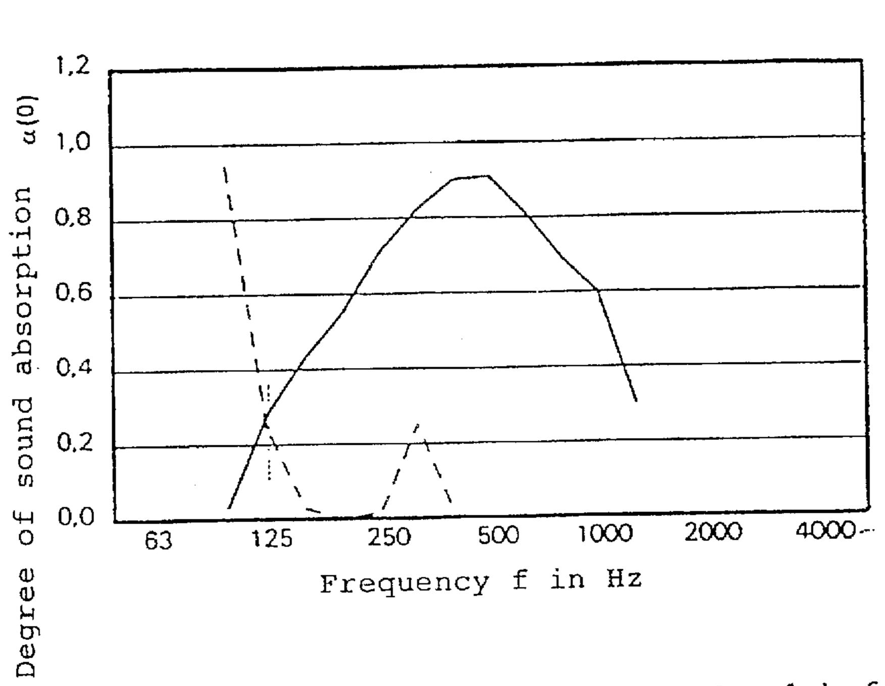
Curve 1: 0.5 mm microperforated steel sheet No. 1 before a 100 mm air space
