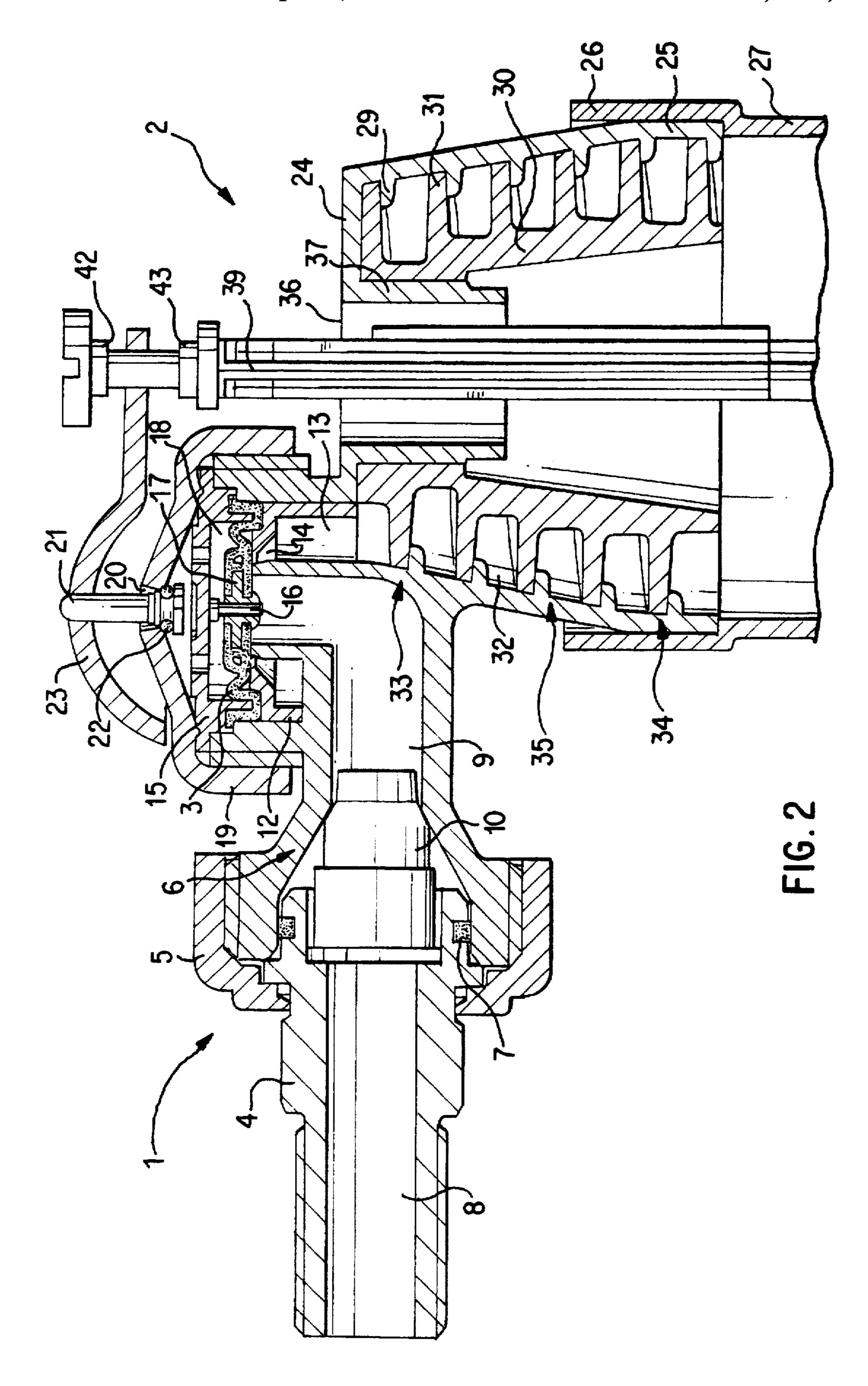
The present invention relates to a WC-cistern filling valve comprising a liquid inlet assigned to a supply line, a liquid outlet assigned to the cistern, and a closing element 5 which is assigned to a valve passage opening arranged between liquid inlet and outlet, and which is switchable by a float according to the filling level in the cistern for opening and closing the valve opening.
