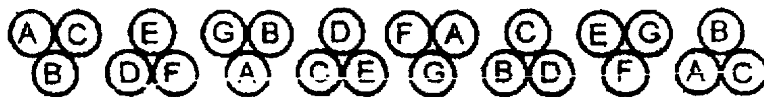
THREADING SEQUENCE FOR THREE COLOR NEEDLE WITH SEVEN COLOR PATTERN
