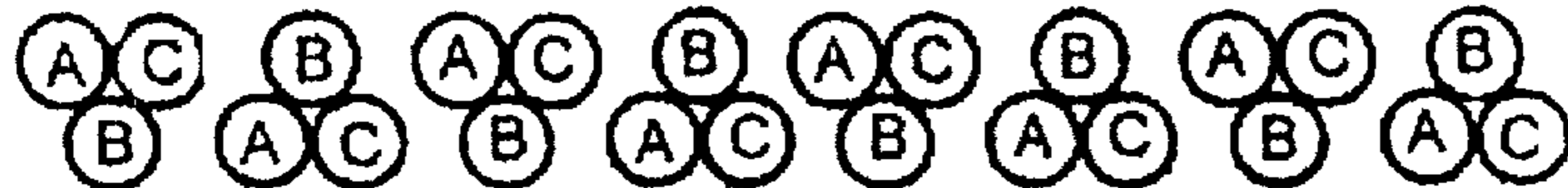
THREADING SEQUENCE FOR THREE COLOR NEEDLE WITH THREE COLOR PATTERN
