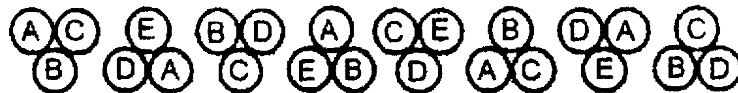
THREADING SEQUENCE FOR THREE COLOR NEEDLE WITH FIVE COLOR PATTERN
