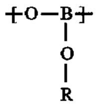
where R is derived from an unsaturated diol or triol. The resin may additionally comprise the units -{O-M-}, where M can vary from one unit to the next and is selected from the group consisting of Si, Ti, Al, Ba, Li, Zr and Hf. Also disclosed is a process for inhibiting the oxidation of carbonaceous materials by impregnating the material with such resins.
