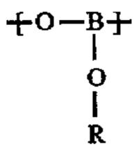
where R is derived from an unsaturated diol or triol.
