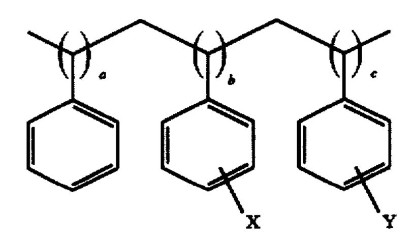
wherein X is selected from the group consisting of —OH, —OCOR, —SH, —SCOR, —CH<sub>2</sub>SH, —CH<sub>2</sub>SCN, —CH<sub>2</sub>SCOCH<sub>3</sub>, —COOH, —COOR, and mixtures thereof, where R is an aliphatic, alicyclic, or an aromatic moiety containing 1 to about 20 carbon atoms;
