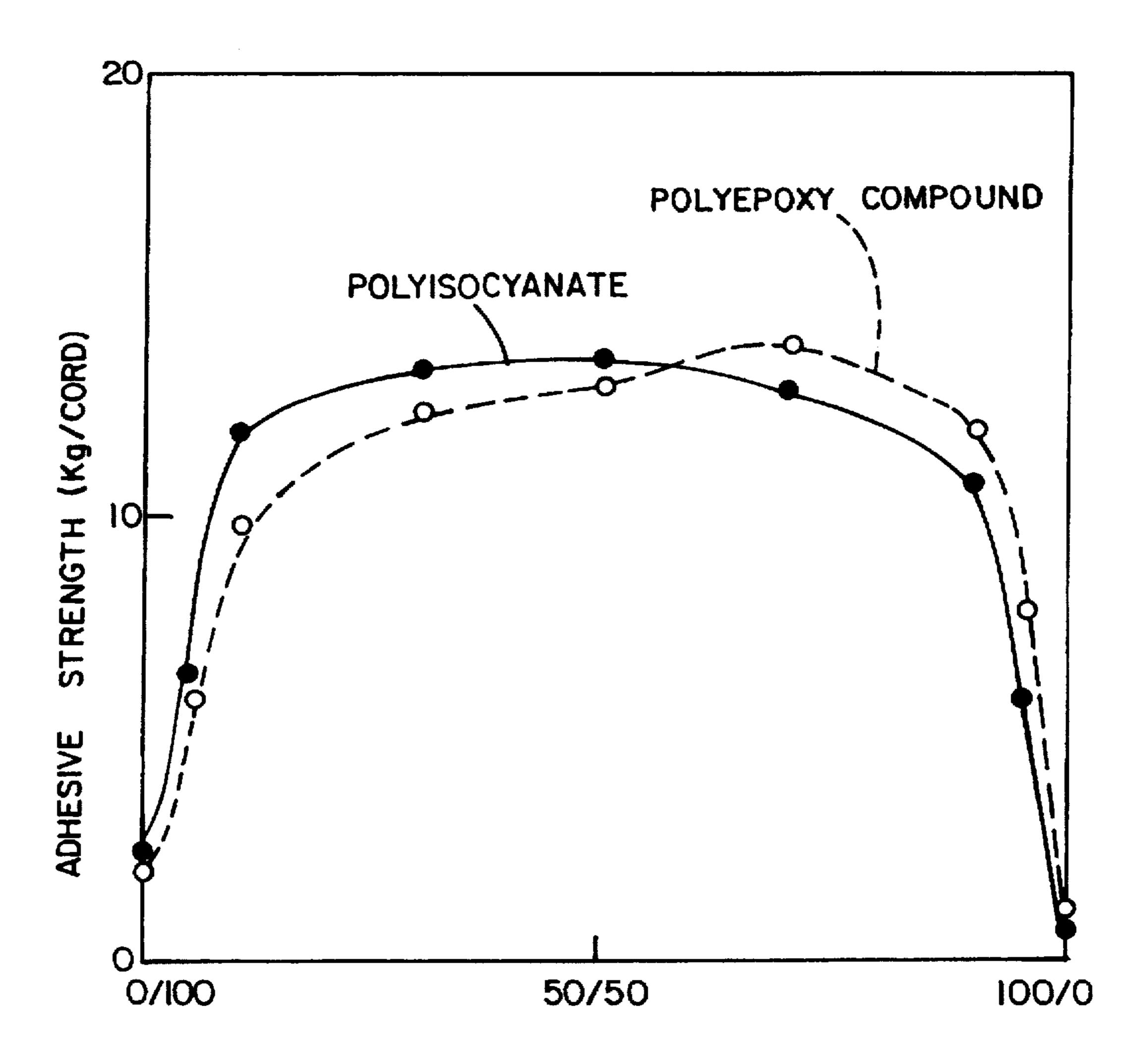
WEIGHT RATIO OF ADHESIVE RUBBER/ POLYISOCYANATE OR POLYEPOXY COMPOUND
