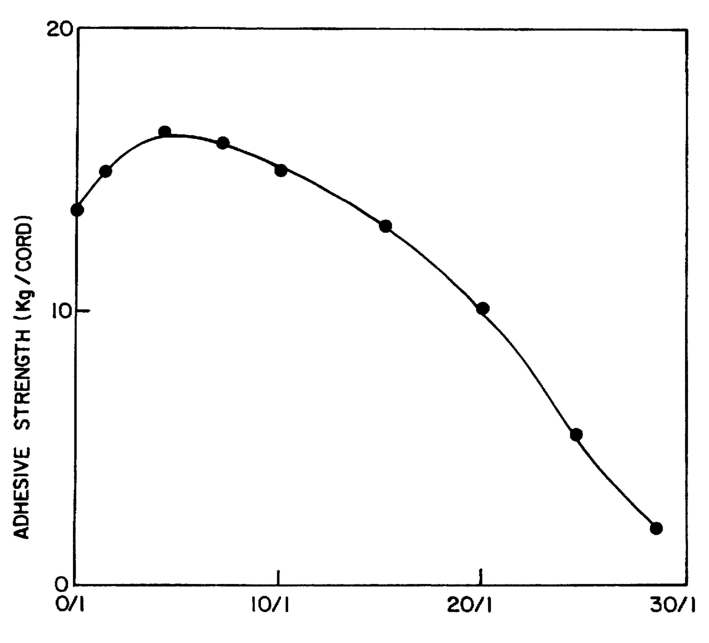
WEIGHT RATIO OF CHLORINATED NATURAL RUBBER / ADHESIVE RUBBER
