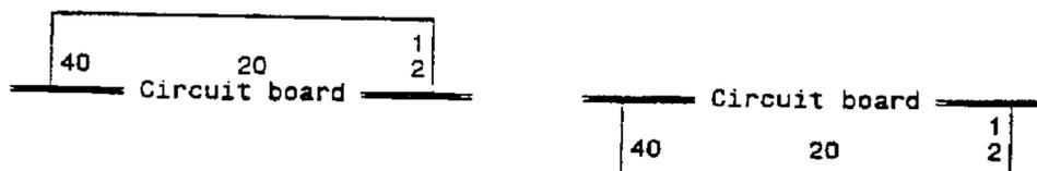
Figure 4 - 40-pin connector mounting
