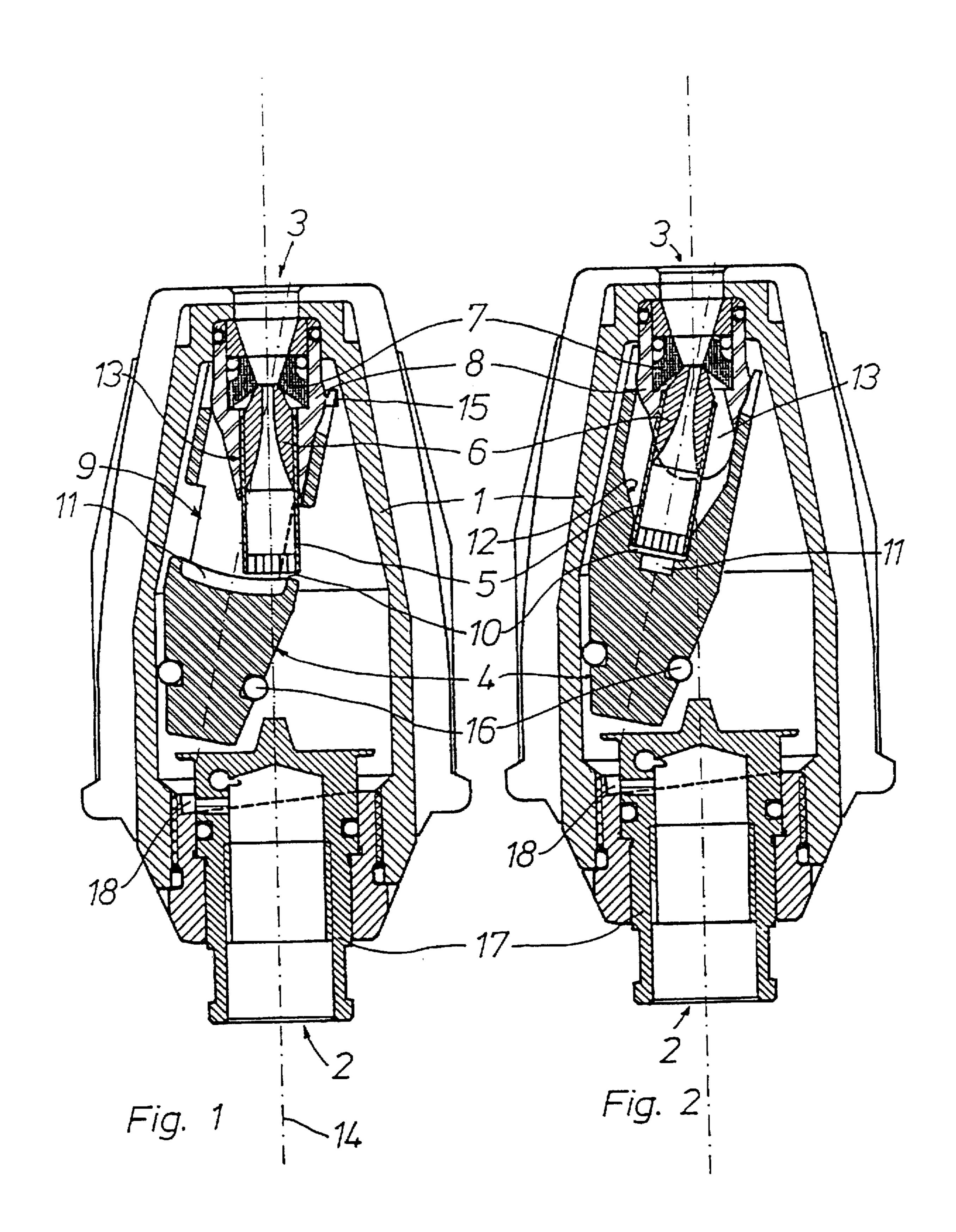
ROTOR NOZZLE, IN PARTICULAR FOR A HIGH PRESSURE CLEANING APPARATUS
