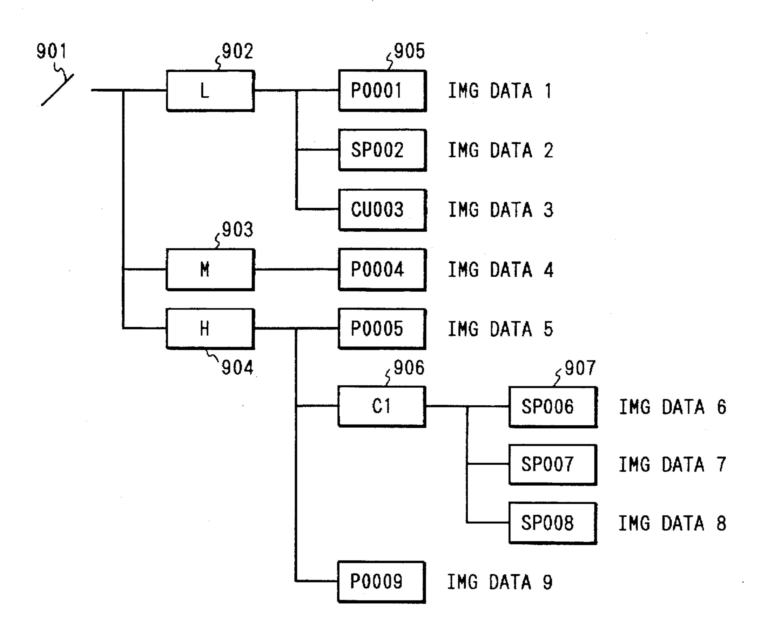
PHOTOGRAPHING-MODE-DEPENDENT IMAGE DATA RECORDING METHOD IN A DIGITAL CAMERA USING HIERARCHICAL STORAGE TO RECORD STILL IMAGES AT A DIFFERENT LEVEL THAN SEQUENTIAL IMAGES
