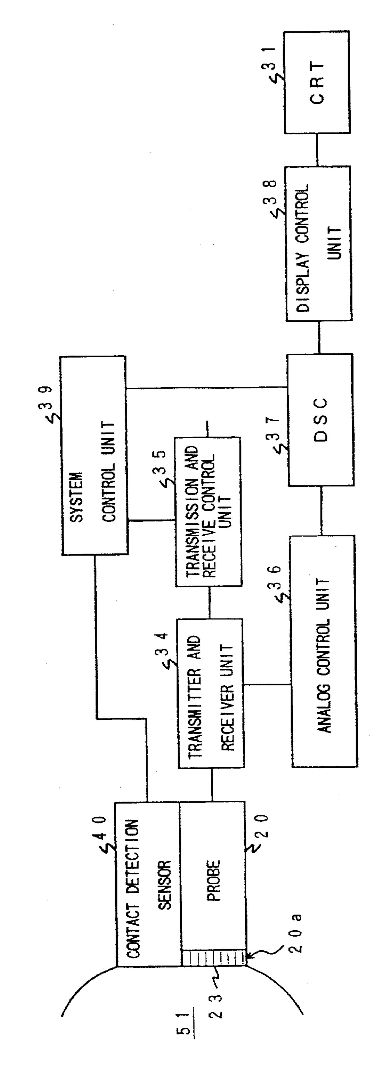
DISPL SYSTEM CONTROL UNIT DSC TRANSMISSION AND RECEIVE CONTROL UNIT 35 39 : MEMORY UNIT IMAGE 34 PROBE
