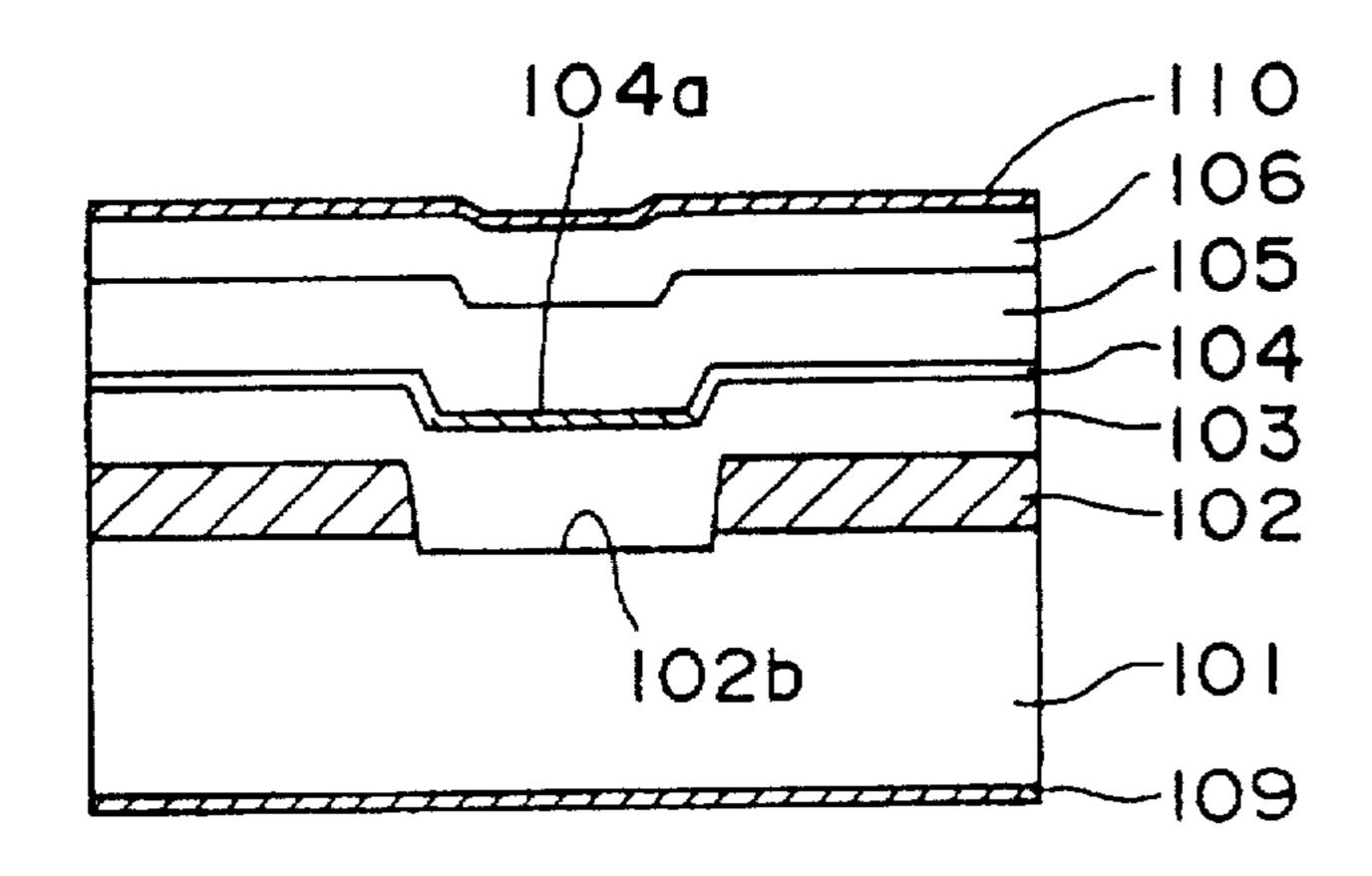
SEMICONDUCTOR LIGHT-EMITTING DEVICE CAPABLE OF HAVING GOOD STABILITY IN FUNDAMENTAL MODE OF OSCILLATION, DECREASING CURRENT LEAKAGE, AND LOWERING OSCILLATION THRESHOLD LIMIT, AND METHOD OF MAKING THE SAME
