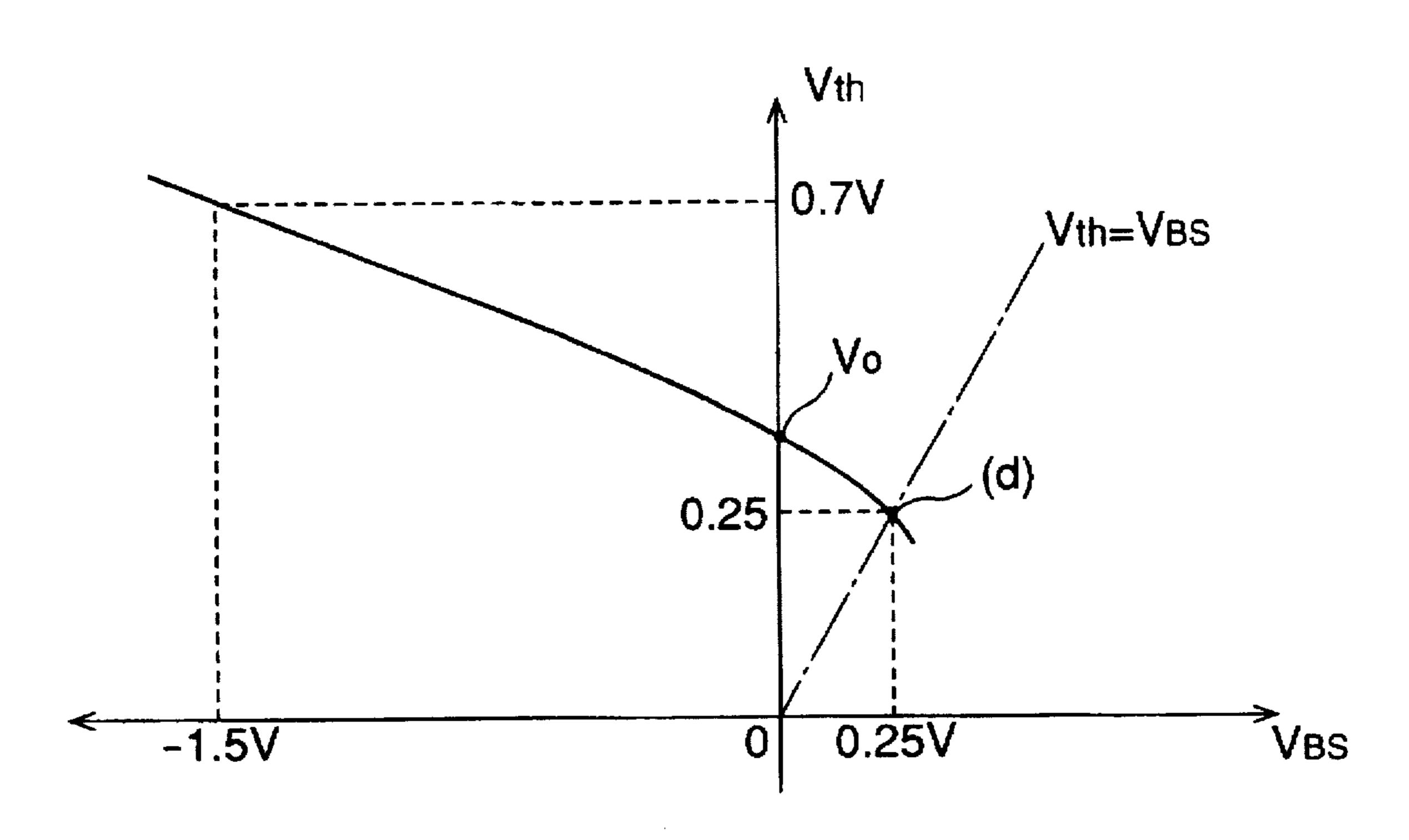
$Vth=V_0+K(\sqrt{2}\phi F+VBS-\sqrt{2}\phi F)$
