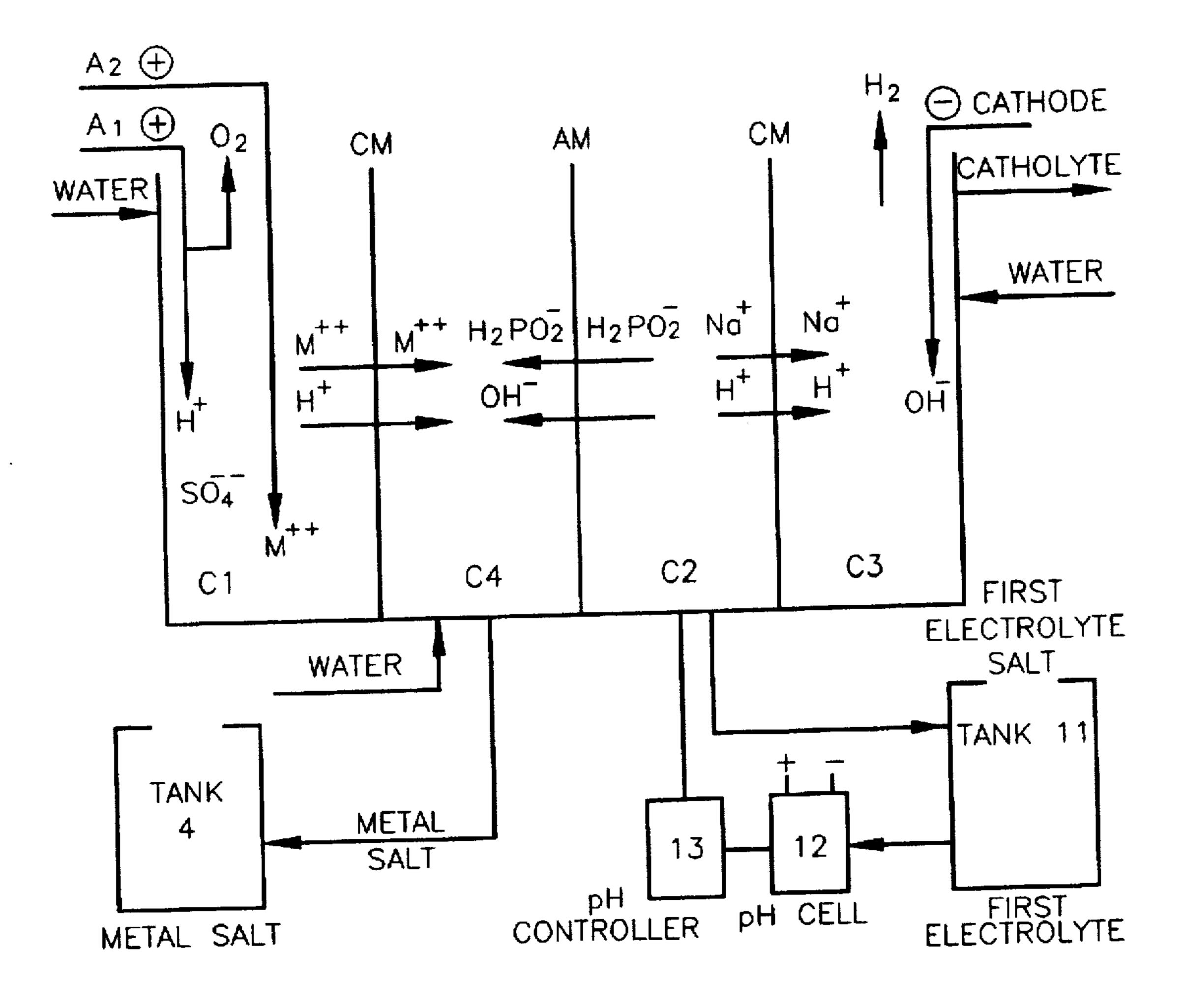
INSOLUBLE ANODE A2 METAL ANODE ANOLYTE COMPARTMENT FIRST ELECTROLYTE COMPARTMENT C3 CATHOLYTE COMPARTMENT C4 SALT FORMING COMPARTMENT METAL CATIONS HYDROGEN ION H2PO2 HYPOPHOSPHITE ANION OH- HYDROXIDE ION Na+ SODIUM ION AM ANION PERMEABLE MEMBRANE CM CATION PERMEABLE MEMBRANE
