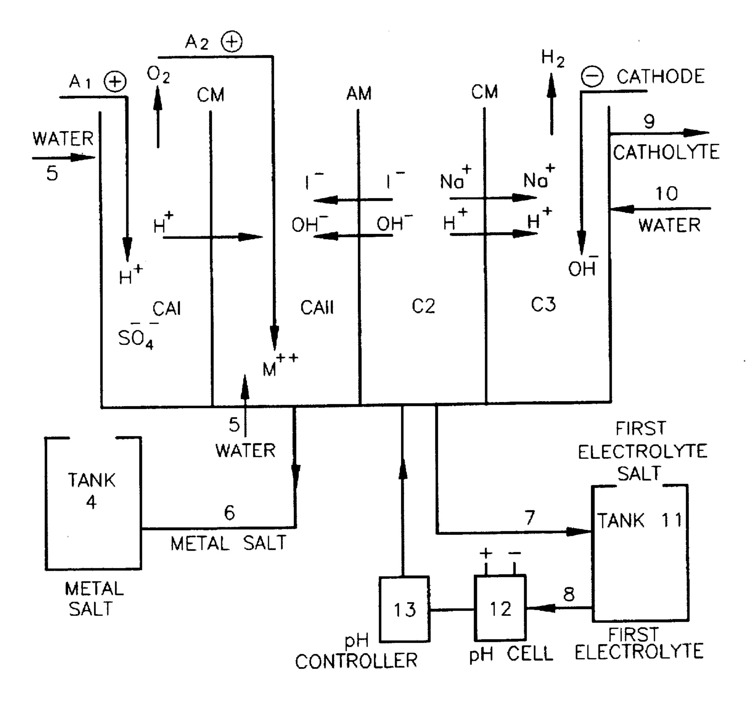
INSOLUBLE ANODE A2 METAL ANODE CAI ANOLYTE I COMPARTMENT CAII ANOLYTE II COMPARTMENT C2 FIRST ELECTROLYTE COMPARTMENT C3 CATHOLYTE COMPARTMENT METAL CATIONS HYDROGEN ION 1 ODINE ION OH HYDROXIDE ION Na + SODIUM ION AM ANION PERMEABLE MEMBRANE CM CATION PERMEABLE MEMBRANE
